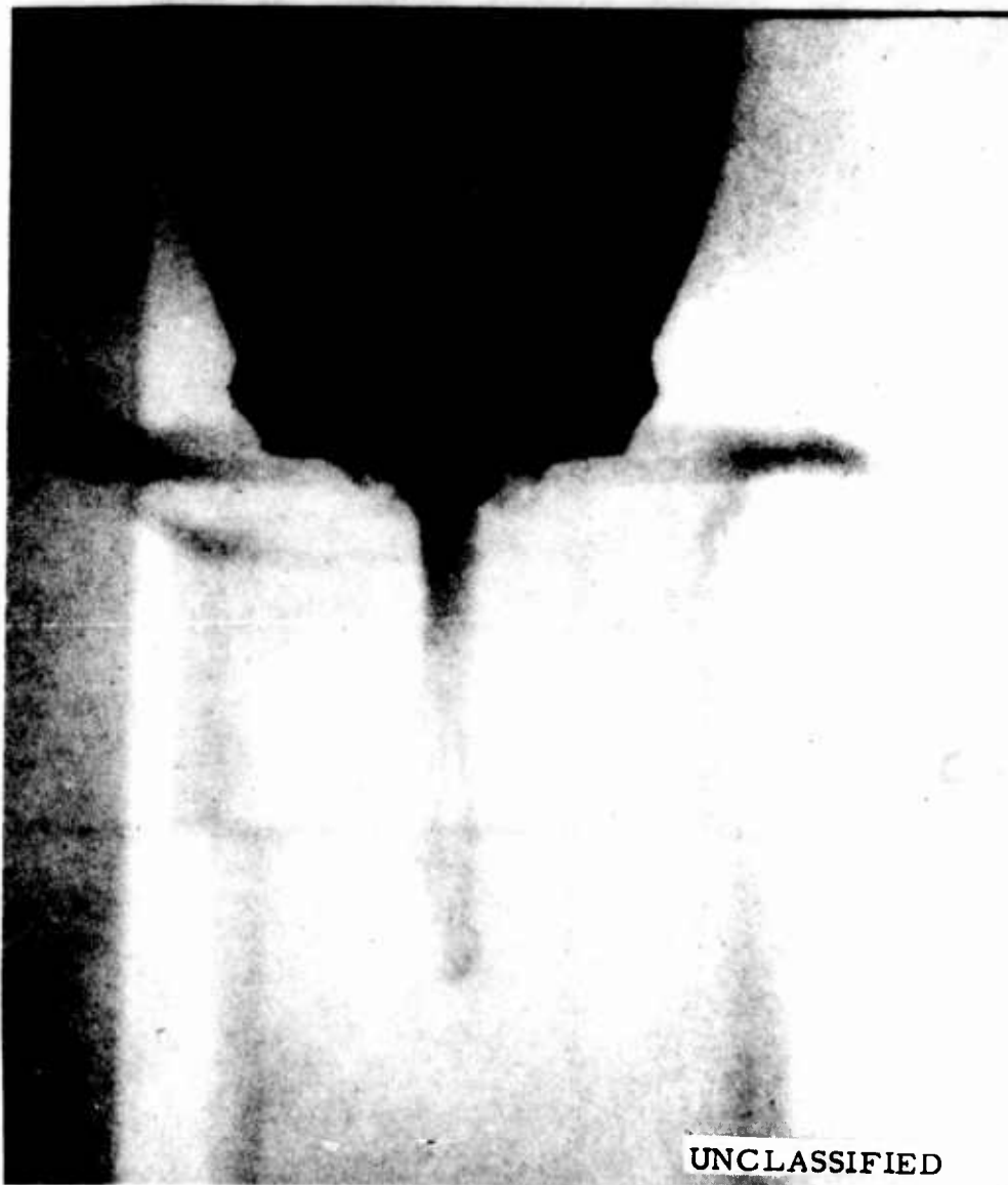
Figure 38. Flash Radiograph of Jet Obtained at Short Standoff From A Precision Shaped Charge Assembly With A Composition B Charge Overdriven by An External PBX 9404 Driver. Note that the Jet is Straight But Badly Disrupted Over the Forward Half, in Contrast With Figure 37.
