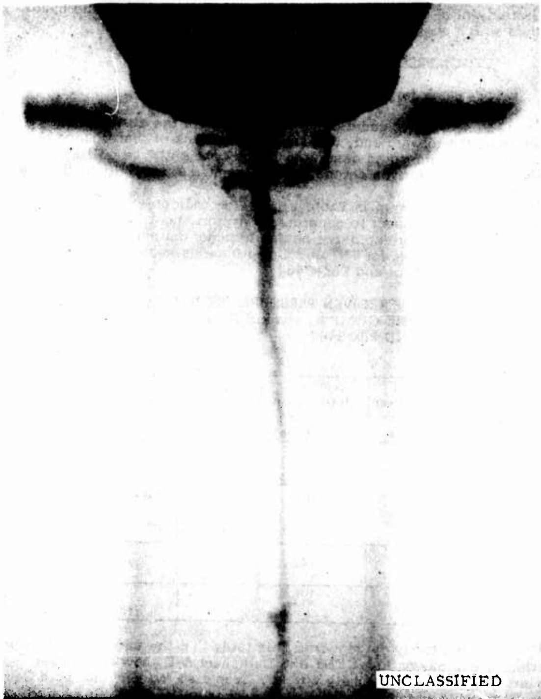
Figure 40. Flash Radiograph of Jet Obtained at Long Standoff From Precision Shaped Charge Assembly with a Composition B Charge Overdriven by an External PBX 9404 Driver. Note that Jet is Straight But Disrupted Over the Forward Half.
