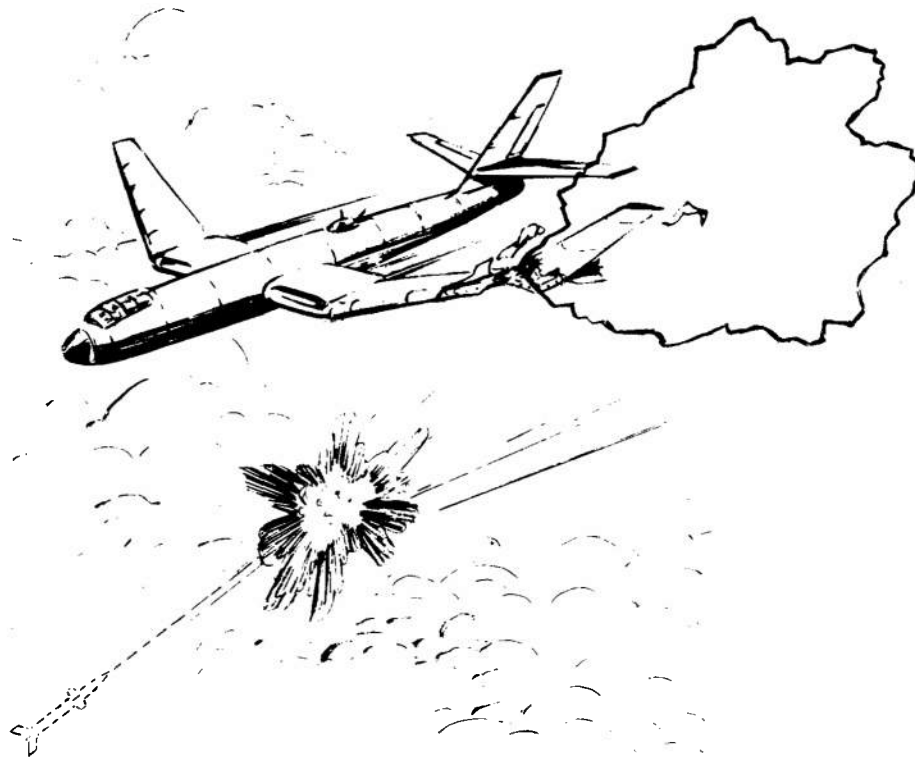
Figure 1-18. Continuous Rod Warhead
