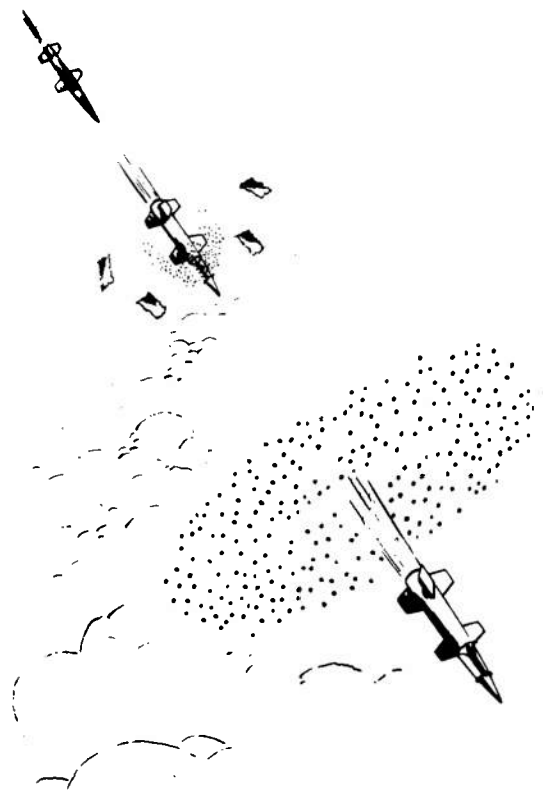
Figure 4-96. Ejection Sequence, Spheres
