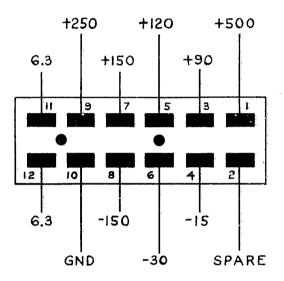
The B+ and bias voltages (except +500) are fed to the power box from a central power supply source located in the basement. The +500 must be supplied by local power supply. The a-c input to the central supplies and the  $\pm 150$ , -15, and -30 outputs are regulated. Heinemann circuit breakers capable of switching in 1 millisecond are used in all lines and are located in remote circuit-breaker boxes. One such box can supply power to as many as six bench power boxes.
