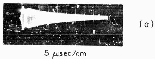
FIG. 11 RF PULSES FROM 6-Mc RING TRANSMITTER SHOWN AT INCREASED SWEEP TIMES
