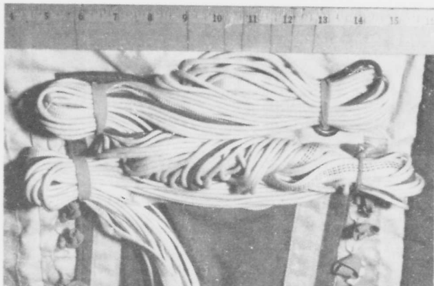
Figure 11 PROCEDURE USED TO STOW SUSPENSION LINES OF PIONEER PARA-COMMANDER MARK I PARACHUTE FOR TWISTED LINE DUMMY DROP TESTS
