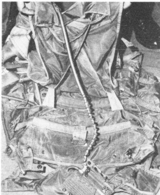
Figure 22 MAJOR DAMAGE TO PIONEER PARA-COMMANDER MARK I PARACHUTE PACK AFTER DROP TEST No. 1023 MADE AT 225 KCAS AND 1000 ft PRESSURE ALTITUDE. NOTE THE TORN FABRIC AND BROKEN MANUAL RIPCORD RELEASE HOUSING.
