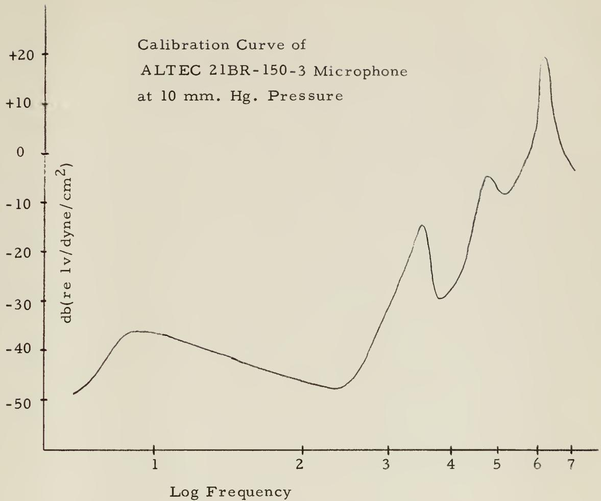
Fig 4. Microphone Calibration Curve
