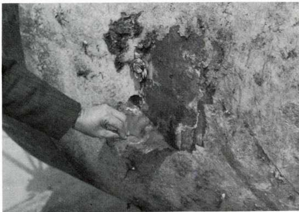
Figure 5-1. Improperly applied vinyl coating being stripped from buoy.
