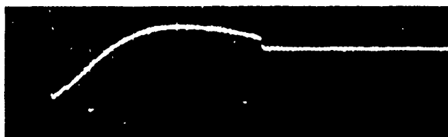
FIGURE 14 Output of \dot{B}_y Coil with Current in Gaussing Loop shown in Fig 13
