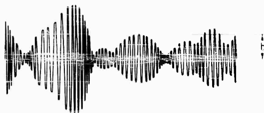
Fig. 5 - Narrow band random acceleration signal and reference acceleration level b (counts made of number of peaks exceeding b )
