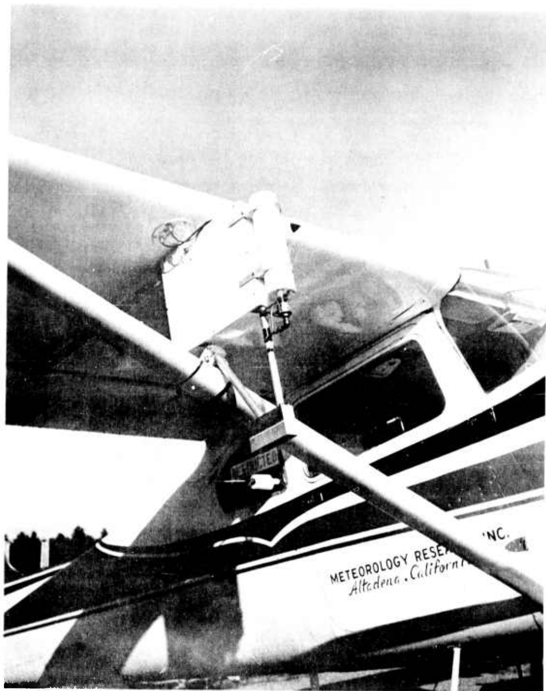
Fig. 1. COATING WHEEL VERSION MOUNTED ON A CESSNA 180.
