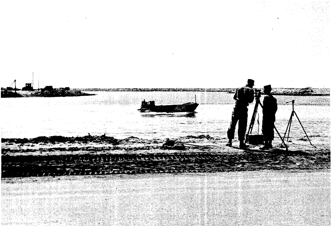
Figure 76. Transit Used To Trace Path of Lighter During Marine Turning Radius Tests.
