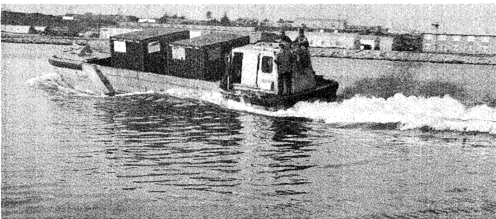
Figure 136. Lighter in Hard-Over Starboard Turn With 10-Ton, 40-Inch-Center-of-Gravity Load and 3, 000 Engine RPM.
