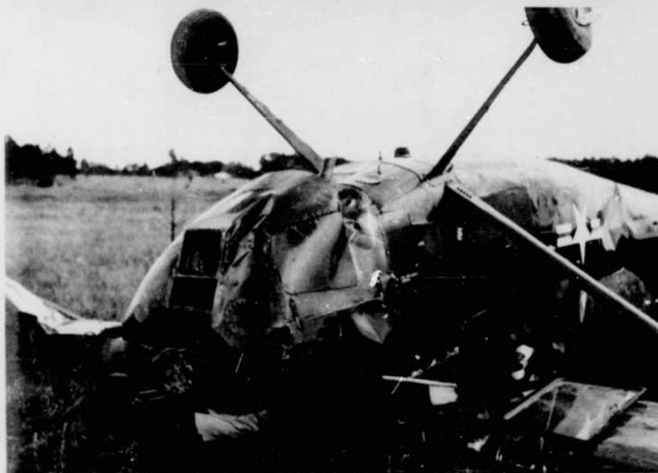
Fig. 6: Typical Groundloop Damage Incurred in Cessna 01 Aircraft Equipped with Standard Landing Gear.
