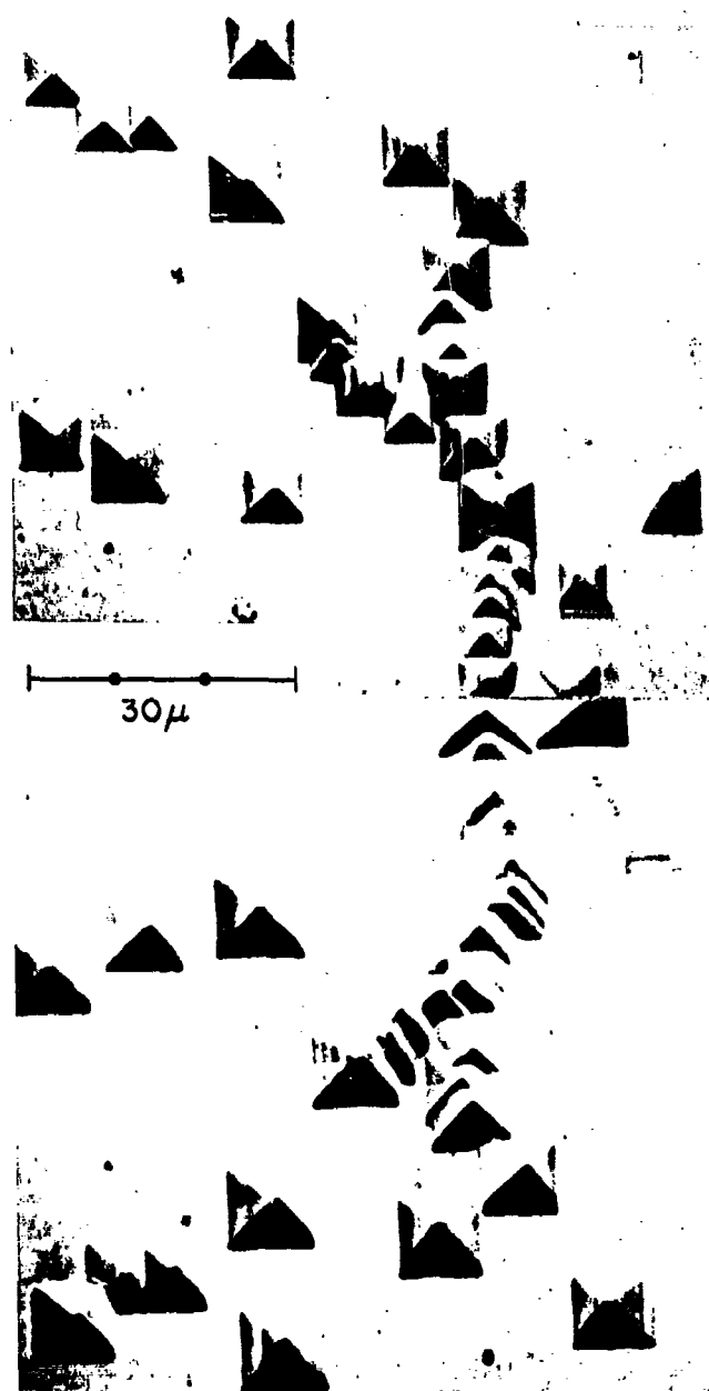
FIG. 4 DISLOCATION ETCH PIT PATTERNS ON THE TWO SURFACES FORMED BY THE CLEAVAGE OF A p-TYPE LEAD TELLURIDE CRYSTAL. THE SURFACE WITH THE SMALLER PITS WAS ETCHED BY HOUSTON AND NORR'S 'IODINE ETCH' AND THE ONE WITH THE LARGER BY THEIR 'IODATE ETCH'.
