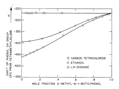
Fig. 6. The proton shift of the phenolic -OH in 2-methyl-6-<u>t</u>-butylphenol, upon dilution, 13 observed at room temperature with a 60 Mc./sec. spectrometer.
