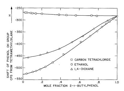
Fig. 5. The proton shift of the phenolic -OH in 2-t-butylphenol, upon dilution, on, observed at room temperature with a 60 Mc./sec. spectrometer.
