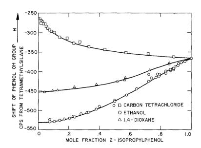
Fig. 3. The proton shift of the phenolic -OH in 2-isopropylphenol, upon dilution, 13 observed at room temperature with a 60 Mc./sec. spectrometer.
