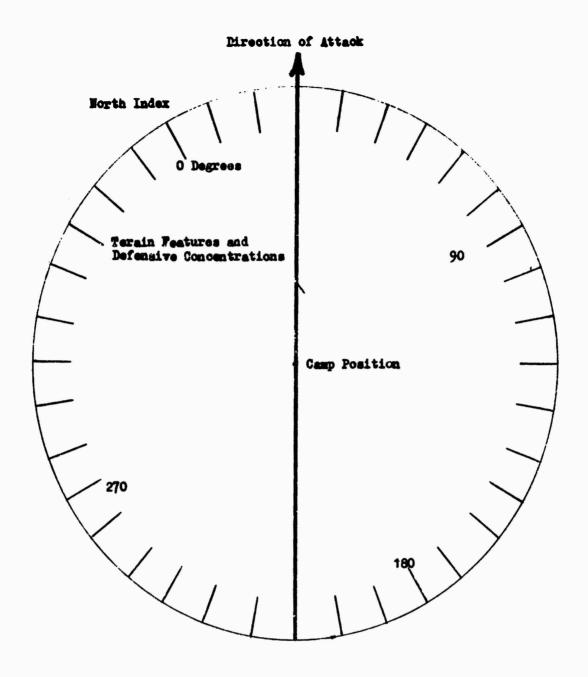
Method of Operation: The target indicator is positioned in asimuth towards North using a permanent indexed reference. The rotating arrow is then positioned toward the direction of attack. Azimuth to target is obtained and a rough range estimation is made. To aid in estimating range and calling for fires, terrain features and defensive concentrations are sometimes indicates on the target indicator with a rough distance scale.
