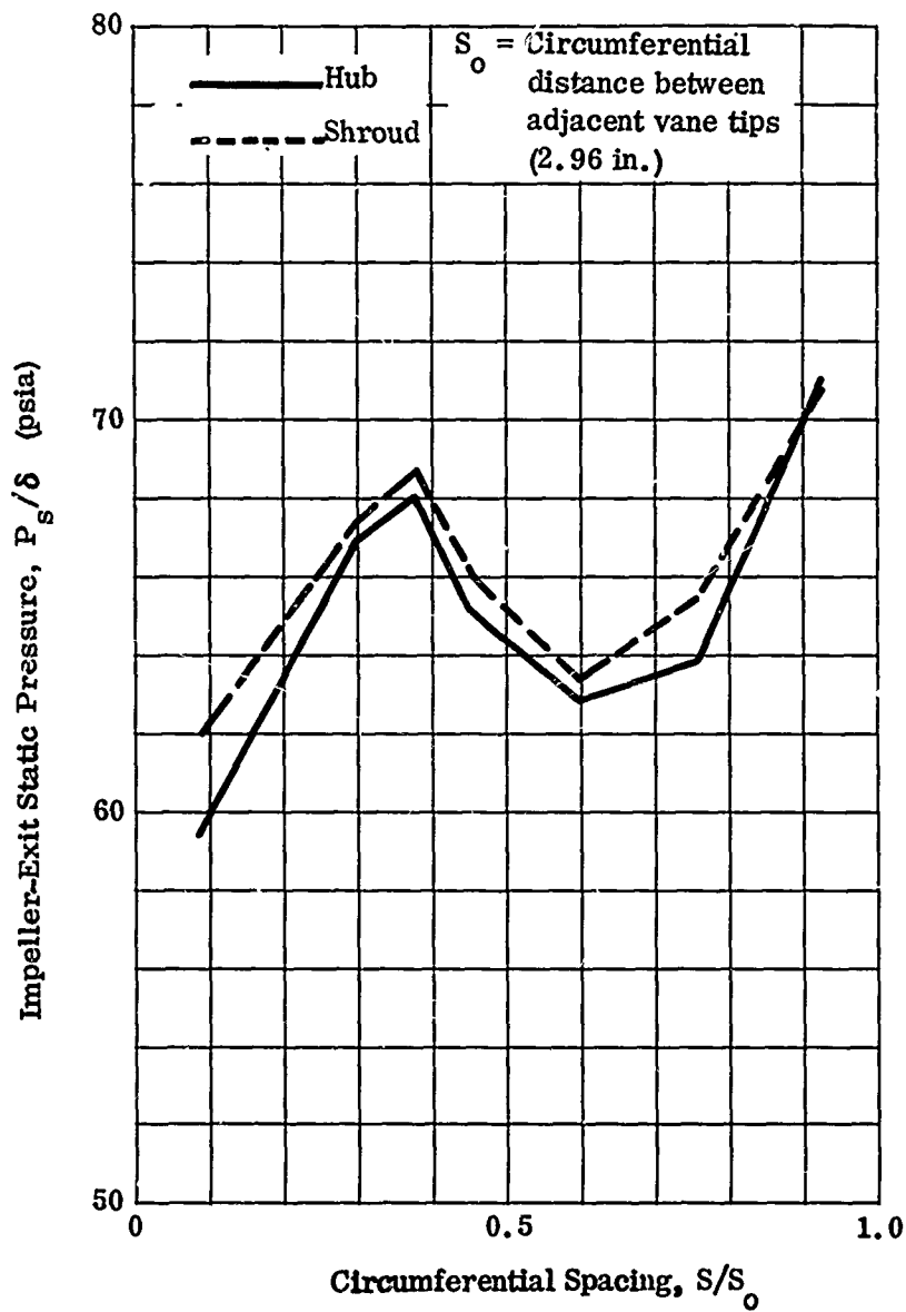
Figure 120. Circumferential Variation of Impeller-Exit Static Pressure.
