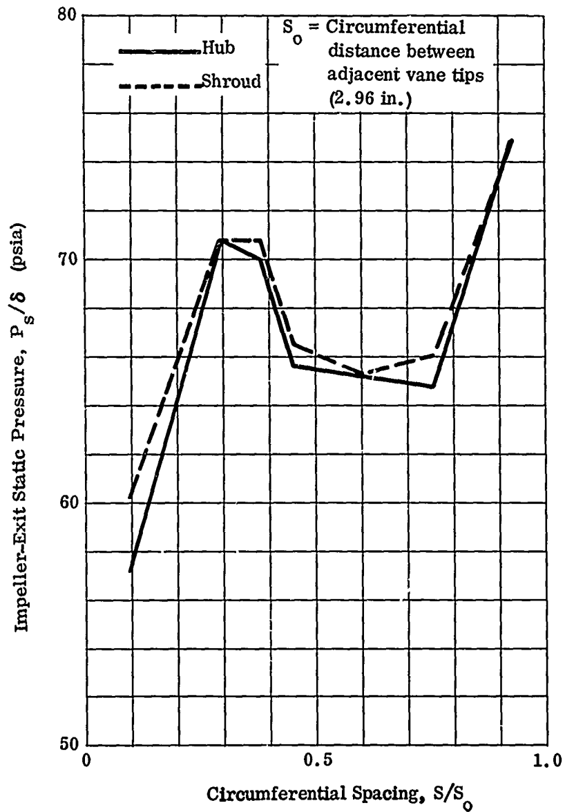
Figure 119. Circumferential Variation of Impeller-Exit Static Pressure.
