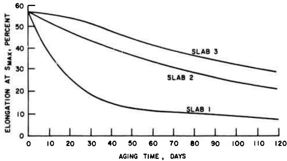
FIG. 7. Tensile Strength and Elongation After Aging at 135°F and 79 Percent Relative Humidity.
