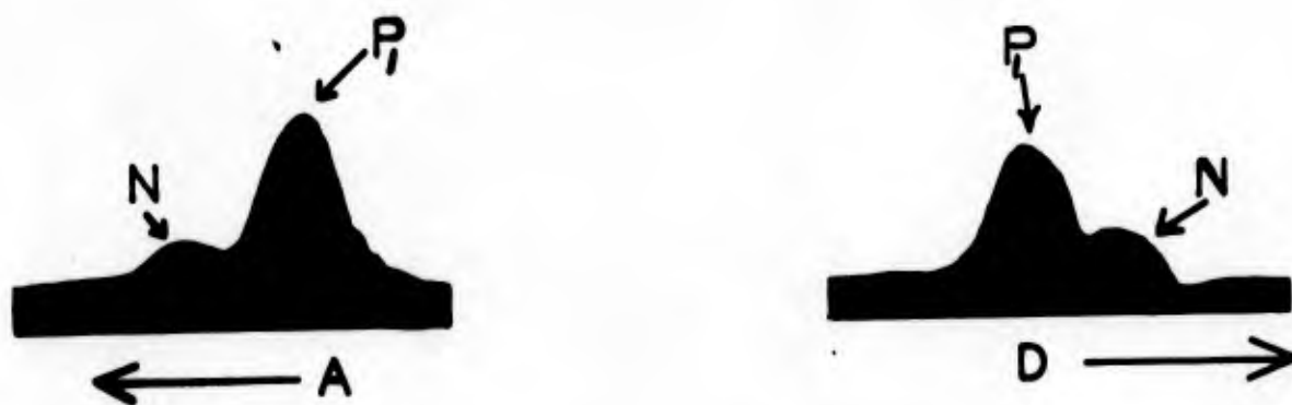
FIG. 50 ELECTROPHORETIC PATTERNS OF FRACTION ULF-15 CACODYLATE BUFFER, pH 7.02 PATTERNS WERE OBTAINED AFTER 2109 SECONDS AT 2.49 VOLTS/CM.
