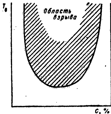
Fig. 4: Ignition point as a function of the percentage composition of the mixture for constant pressure. Top: "explosive region".
