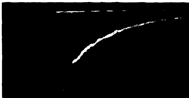
(a) Glass #3 Nd F 3 Sweep speed 200 \mu sec/div approx decay time 580 \mu sec
