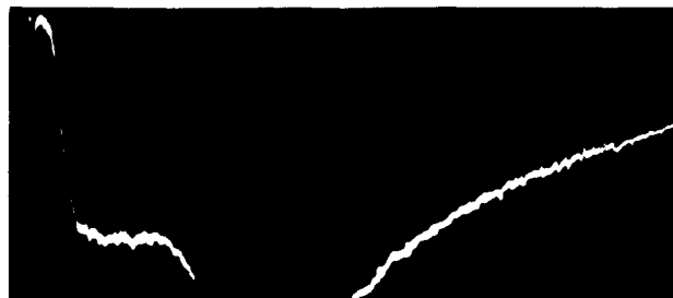
(c) Flash tube at 3.1 kv Capacitance 100 \mu fd Amp sensitivity 0.5v/cm Sweep speed 100 \mu sec/div Photomultiplier at 1 kv
