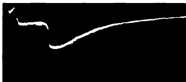
FIG. 6.1 OSCILLOSCOPE TRACE OF OUTPUT FROM NEODYMIUM DOPED GLASS LASER. DOPING LEVEL IS 2 PERCENT. HOST IS GLASS No. 3. LASER WAS OPERATED AT ROOM TEMPERATURE.
