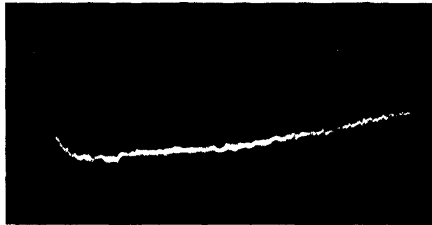
(a) Flash tube at 2.4 kv Capacitance 100 \mu fd Amp sensitivity 0.5v/cm Sweep speed 100 \mu sec/div Photomultiplier at 1 kv
