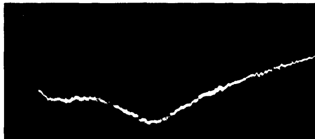
(b) Flash tube at 2.8 kv Capacitance 100 \mu fd Amp sensitivity 0.5v/cm Sweep speed 100 \mu sec/div Photomultiplier at 1 kv
