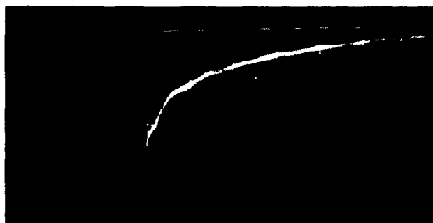
(b) Glass #4 Nd F 3 Sweep speed 200 \mu sec/div approx decay time 440 \mu sec
