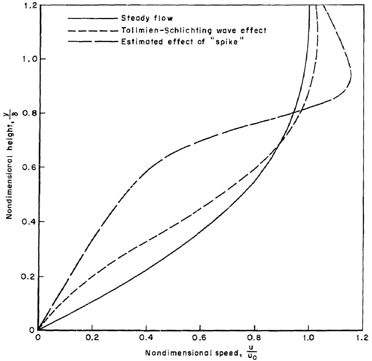
Fig.2—Speed distribution in the laminar boundary layer on a flat plate
