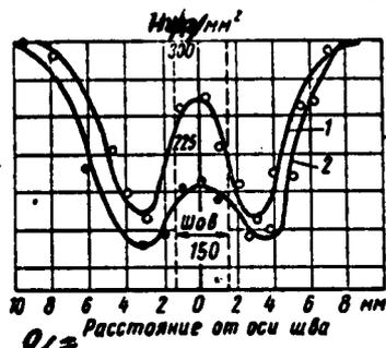
Fig. 4. Hardness of welded joint made of tantalum with thicknesses of 1 mm made with tungsten (1) and tantalum (2) electrode; a-distance from axis of seam
