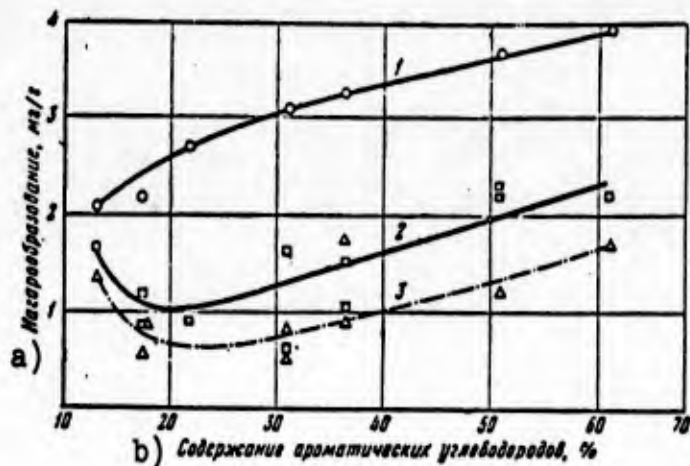
Fig. 94. Variation of scaling as a function of aromatic-hydrocarbon content in fuel and additives to fuel. 1) Without additives; 2) additive A; 3) additive B. a) Scaling, mg/g; b) aromatic-hydrocarbon content, %.
