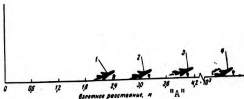
Fig. 62. Takeoff characteristics of a turbojet bomber over a 3-meter obstacle. 1) 60%-magnesium suspension in the afterburner + injection of water; 2) 60%-magnesium suspension in afterburner; 3) conventional fuel in afterburner; 4) no increase in thrust due to augmentation in afterburner; A) take-off distance, m.
