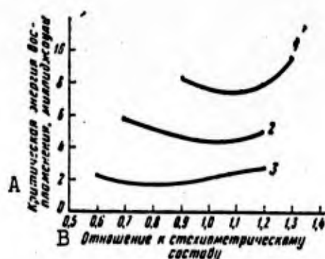
Fig. 100. Effect of degree of hydrocarbon saturation on critical electric-spark ignition energy for combustible mixture. 1) Ethane; 2) ethylene; 3) acetylene. A) Critical ignition energy, millijoules; B) ratio to stoichiometric composition.
