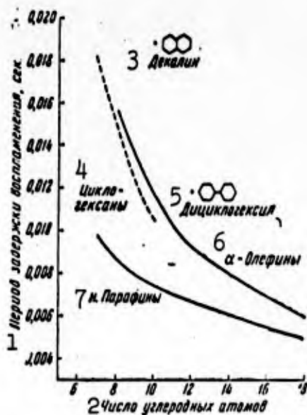
Fig. 107. Ignition lag for hydrocarbons in a bomb at 582° and 21.1 atm. 1) Ignition lag, sec; 2) number of carbon atoms; 3) decalin; 4) cyclohexanes; 5) dicyclohexyl; 6) α-olefins; 7) n. paraffins.
