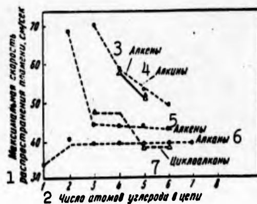
Fig. 118. Influence of hydrocarbon structure and molecular weight on maximum velocity of flame propagation in hydrocarbons mixed with air. 1) Maximum flame-propagation rate, cm/sec; 2) number of carbon atoms in chain; 3) alkenes; 4) alkynes; 5) alkenes; 6) alkanes; 7) cycloalkanes.
