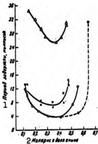
Fig. 136. Ignition lag of trialkyl amines with nitric acid in bomb as function of mole fraction of amine. 0) Triethylamine, bomb filled with air; ●) triethylamine, bomb filled with oxygen; \Delta ) tributylamine; x) tripropylamine. 1) Ignition lag, millisecc; 2) mole fraction of amine.
