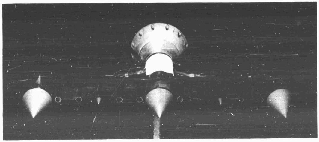
Fig. 5.12 Calibration rake (From Ref. 5.10)
