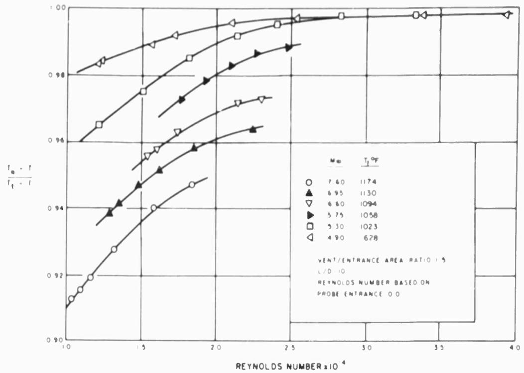
Fig.1.7 Variation of probe temperature recovery factor with free-stream Reynolds number at various free-stream Mach numbers (From Ref.1.3)
