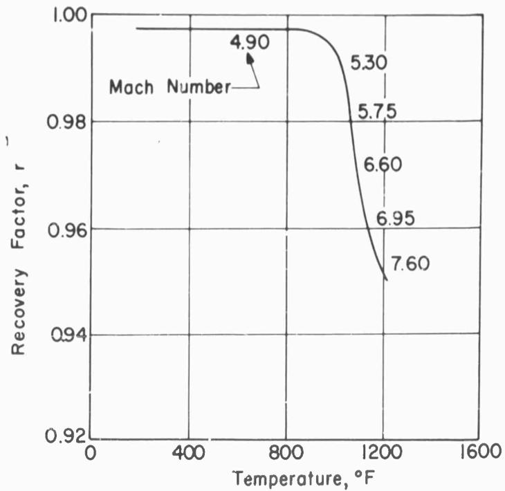
Fig.1.8 Fall-off of recovery factor with temperature and (secondarily) Mach number. Single-shielded probe, RN = 20,000 (Cross-plot from Fig.1.7)
