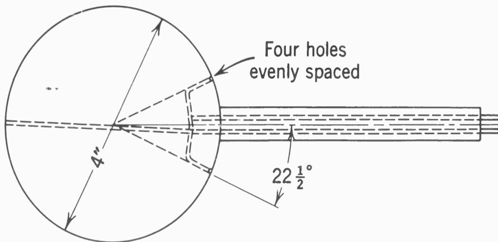
Fig.2.14 Turbulence sphere for a 100 m.p.h. tunnel
