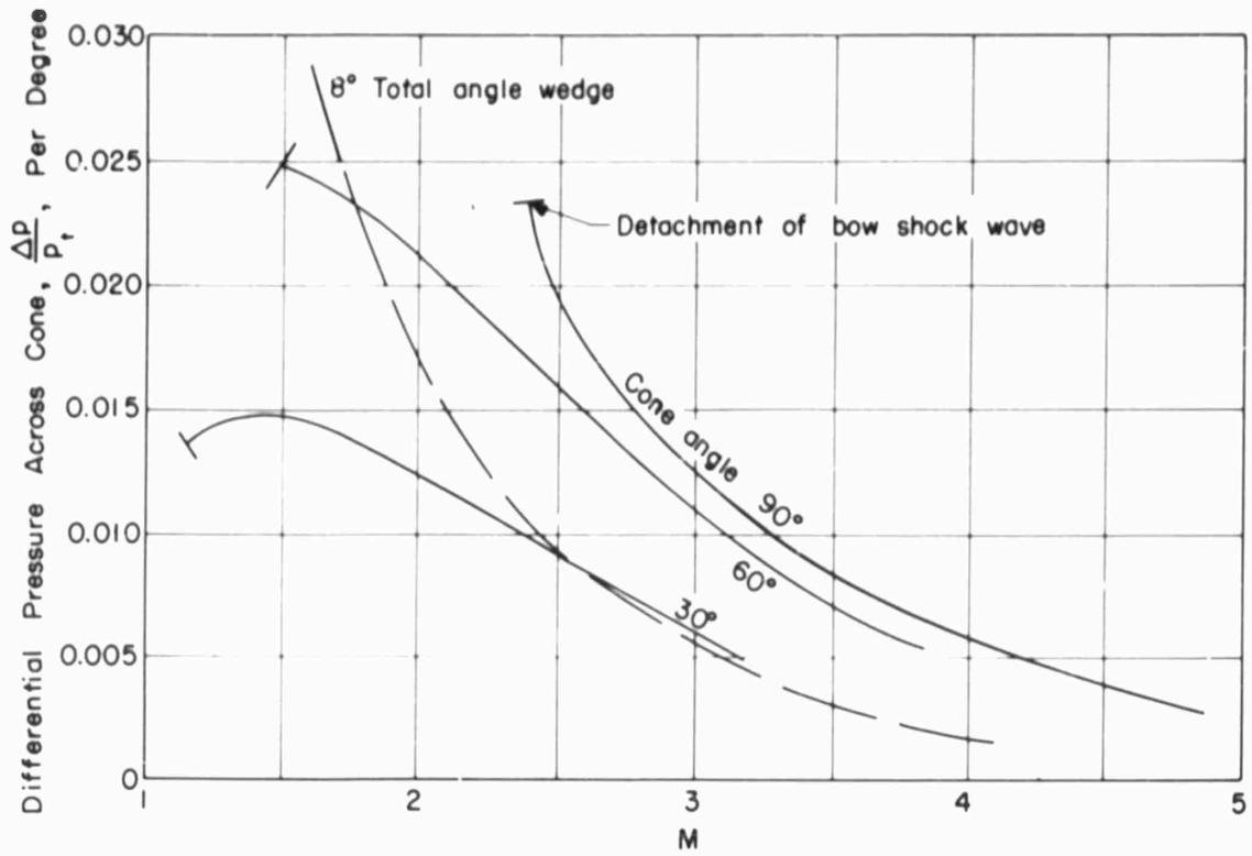
Fig.5.10 Sensitivities of several yawmeters at supersonic speeds, pressure ratio per degree
