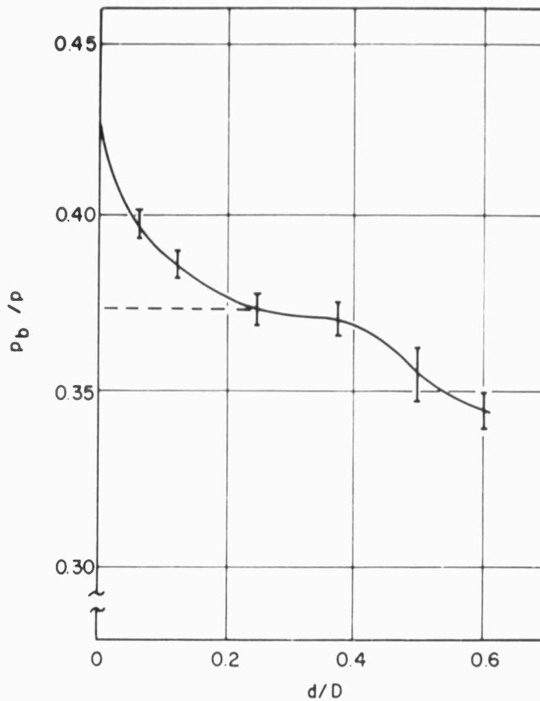
Fig. 7.3 Effect of sting to model diameter ratio on base pressure of an ogive-cylinder model;  $RN = 15 \times 10^6$ , turbulent boundary layer,  $M = 2.97$  (Redrawn from Ref. 7.7)
