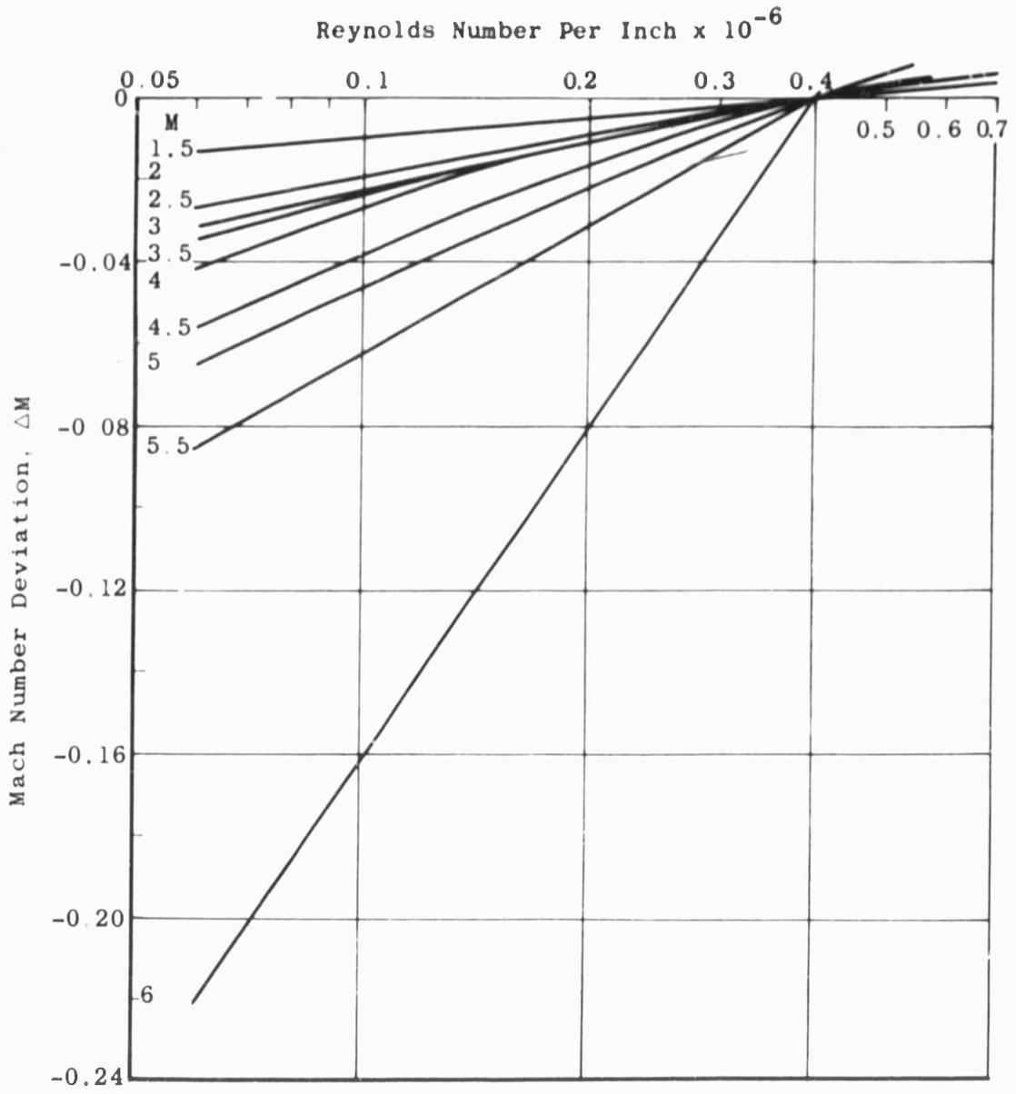
Fig.5.5 Variation of centerline Mach number with Reynolds number, 40 inch tunnel
