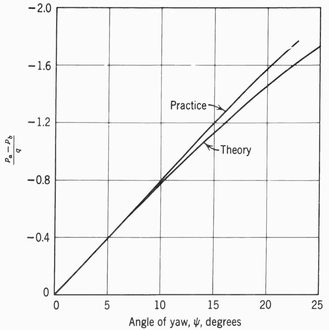
Fig.2.12 Calibration curves for the yawmeter in Fig.2.11
