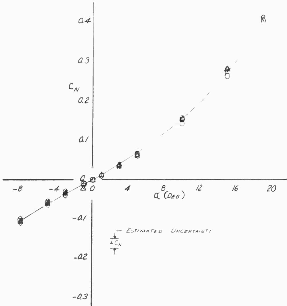
Fig.6.3 The negligible effect of liquefaction on the normal force coefficients of an AGARD Model B;  $M = 8.0$  (From Ref.6.2) ('ppm' equals parts per million)
