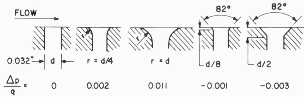
Fig.2.6 Static pressure error due to hole size and lip shape,  $M = 0.4$  to  $0.8$
