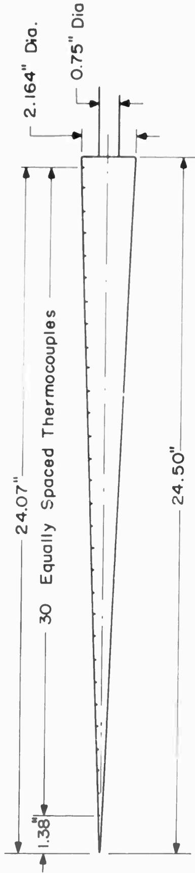
Fig. 5.13 Dimensions of JPL transition cone (From Ref. 5.12)
