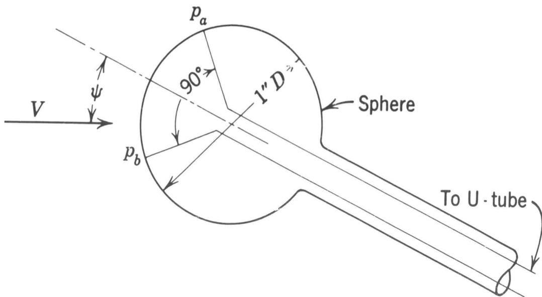
Fig.2.11 Spherical yawmeter
