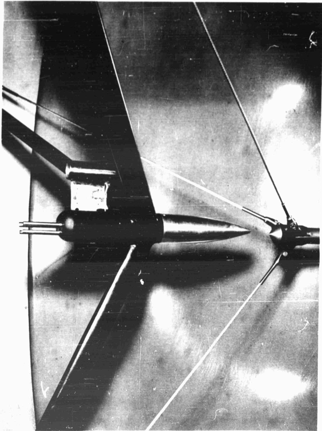
Fig.4.2 Total-head tubes (four) and shielded stagnation-temperature probe in a settling chamber. The extra total-head tubes are to reduce fill time when several multi-manometers are used and  $p_t$  is a reference pressure. The cable-mounted rig at right was for a special test
