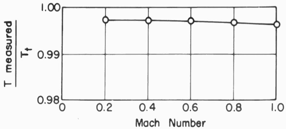
Fig.2.7 Effect of Mach number on temperature recovery ratio of single-shielded probe;  $p_t = 2900 \text{ lb/in.}^2$ ,  $T_t = 140^\circ\text{F}$ ; tube diameter = 0.12 inch
