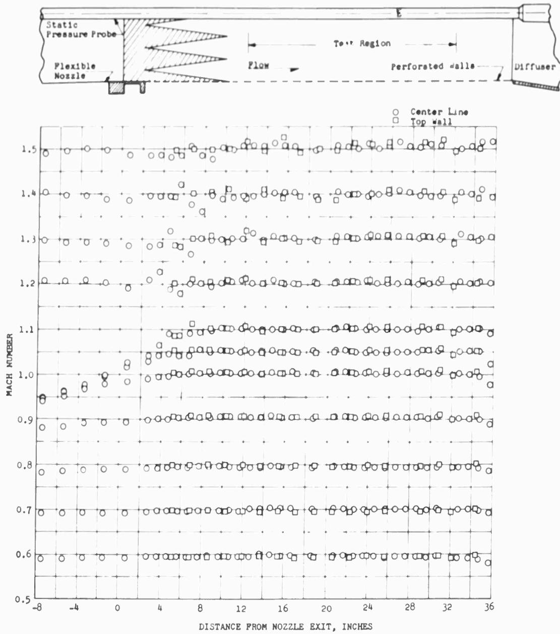
Fig.4.6 Calibration plots for a transonic tunnel. The circles are from the static pipe readings; squares are from wall pressure taps (From Ref.4.4)
