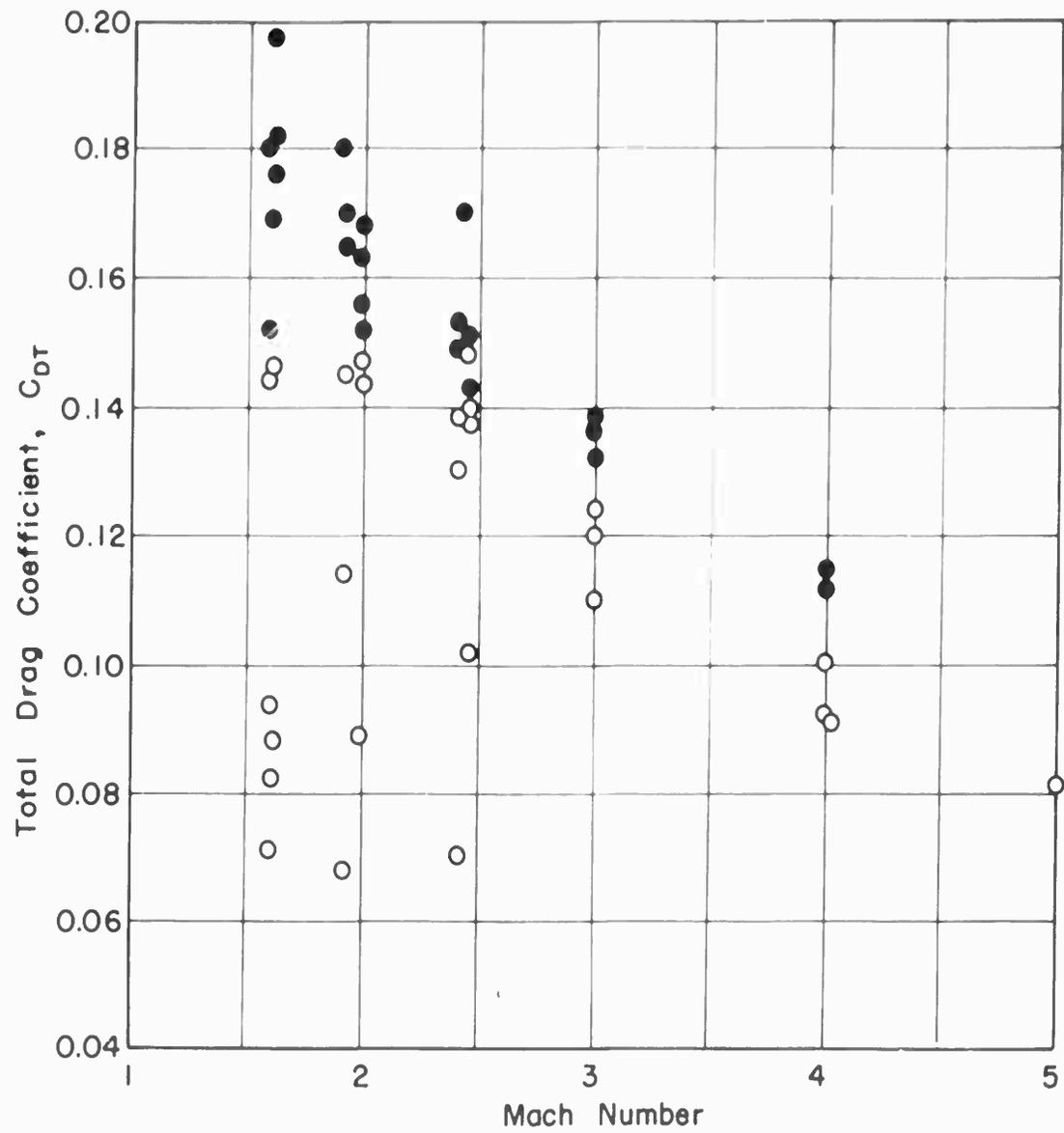
Fig.7.5 Wind tunnel tests of AGARD Model A under a wide range of Reynolds numbers (from  $4$  to  $29 \times 10^6$ ); solid symbols have fixed transition; Figure redrawn from Ref.7.10, data from AEDC and NASA tests
