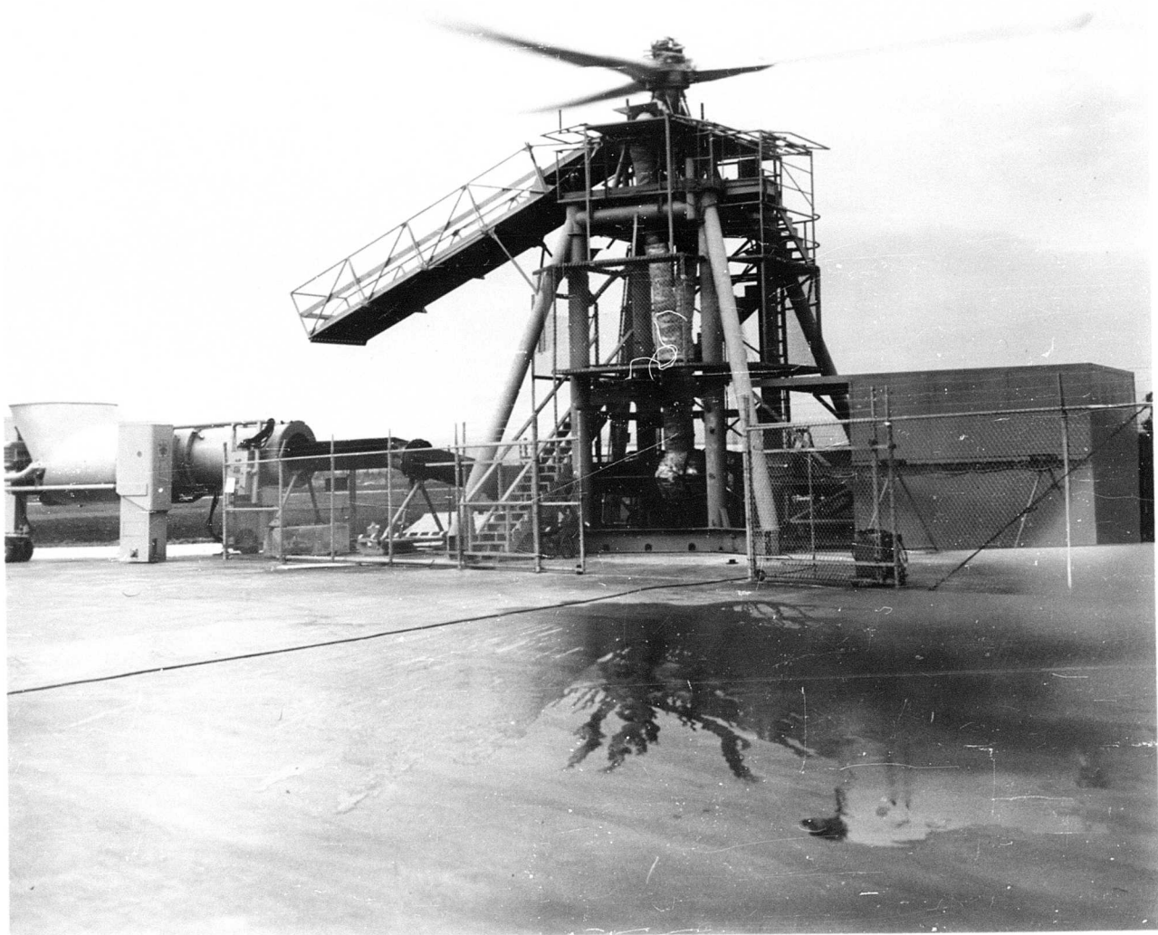
Hot Cycle Rotor Undergoing Whirl Test
