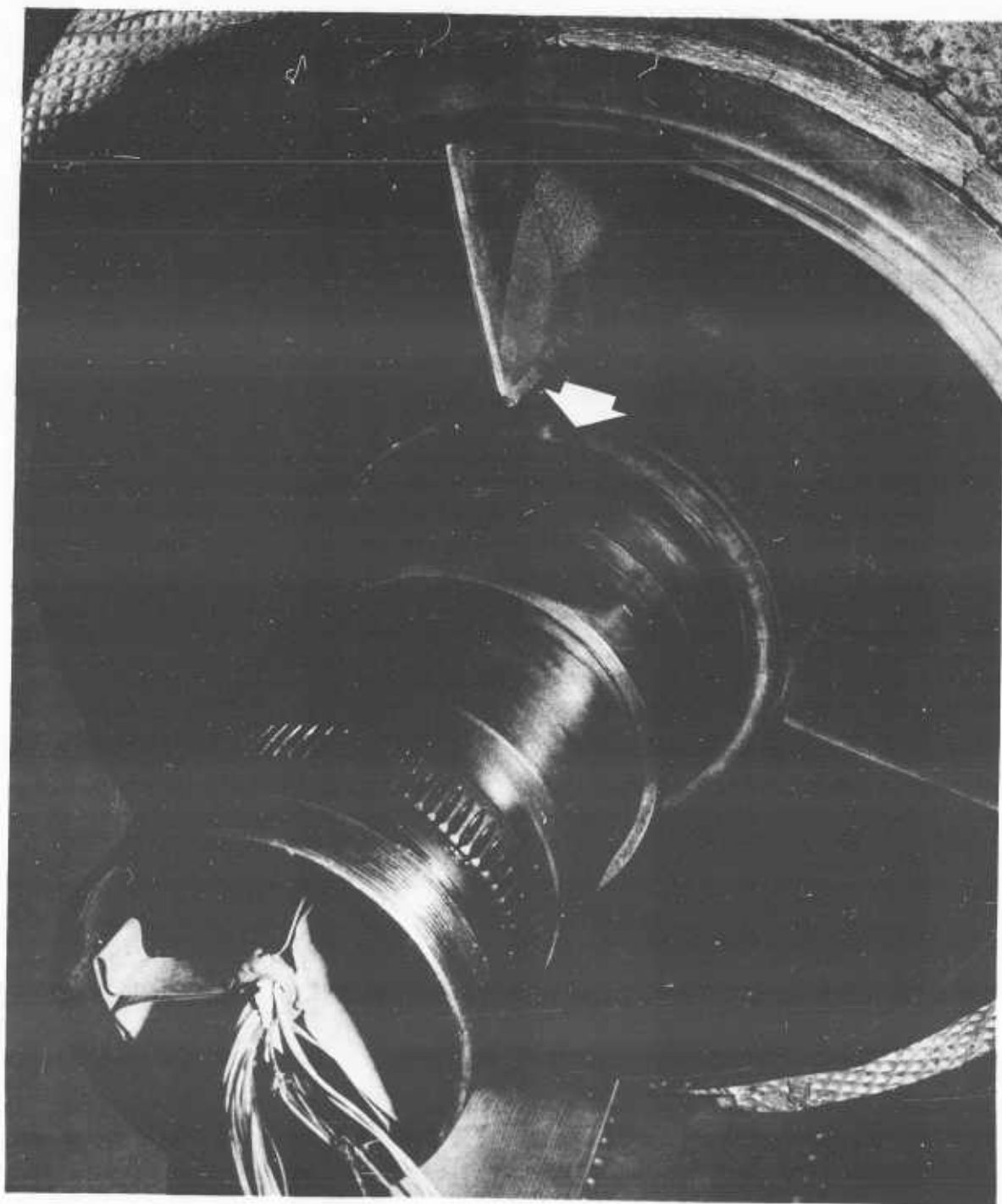
Figure 5.6-8 Hub Upper Duct and Seal Faces After 18 Hours. Note apparent sub-surface corrosion under aluminum oxide plating.
