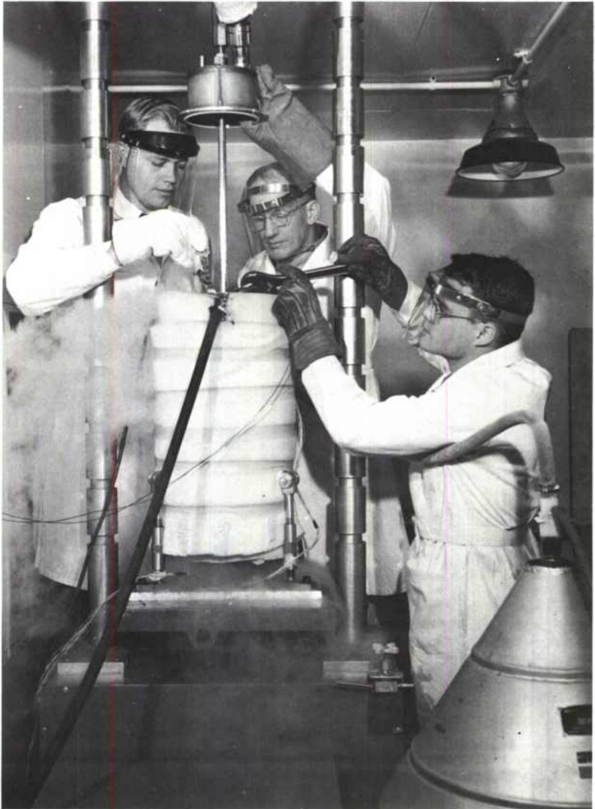
Figure 18. Liquid-Hydrogen Test Chamber Being Prepared for Test
