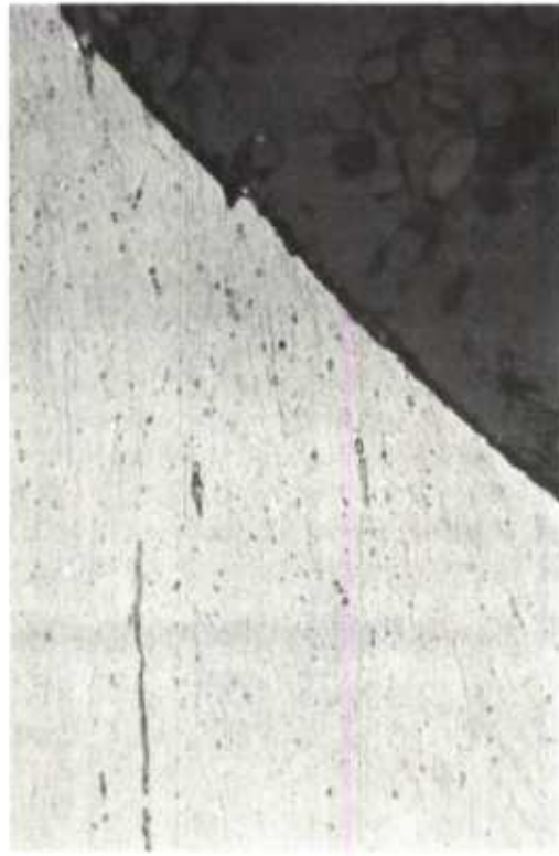
Base Metal 500X -100° F Oxalic Electrolytic Etchant
