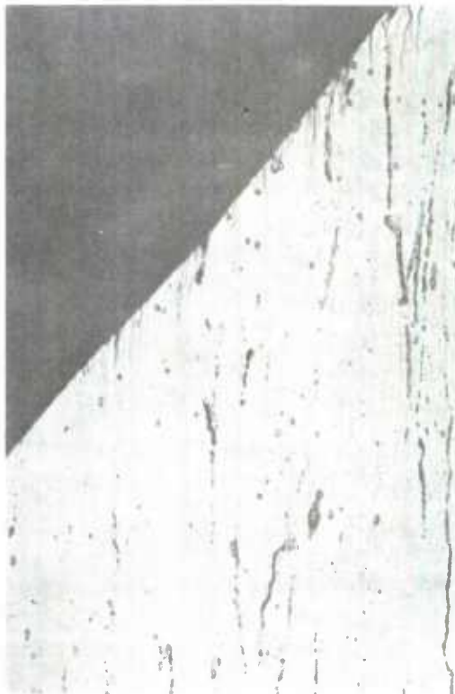
Base Metal 500X -423°F Oxalic Electrolytic Etchant
