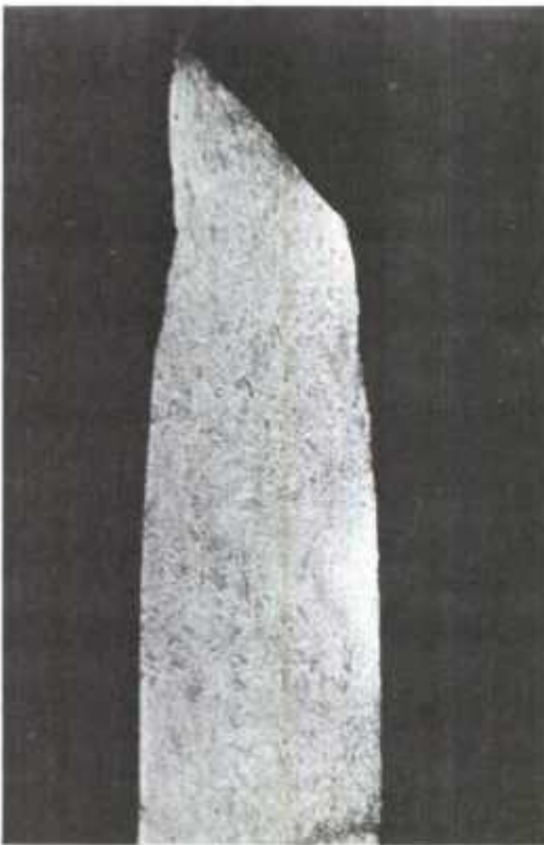
Weld 50X 78°F Oxalic Electrolytic Etchant
