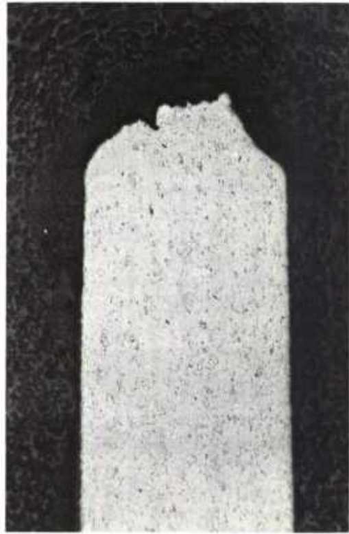
Base Metal 50X -320° F Kroll's Etchant
