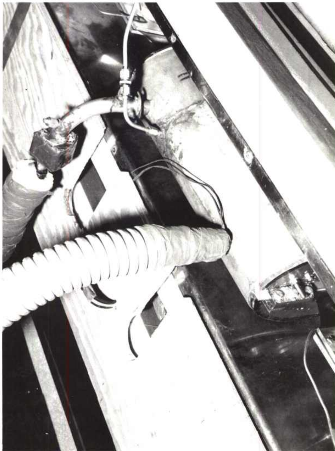
Figure 26. Fatigue Test Bed with Liquid-Hydrogen Test Chamber
