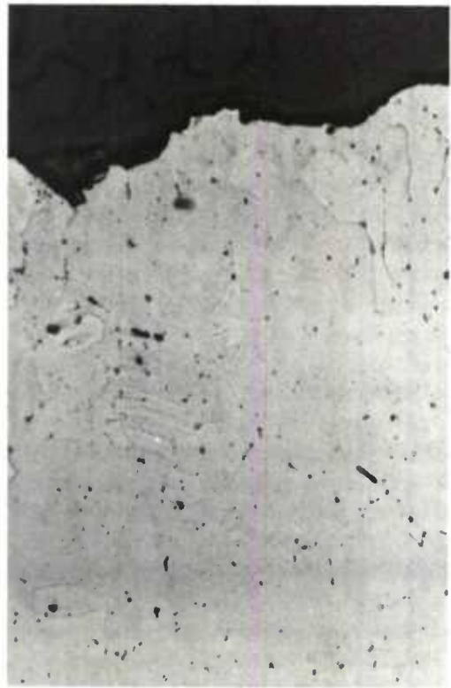
Base Metal 500X -423° F Kroll's Etchant
