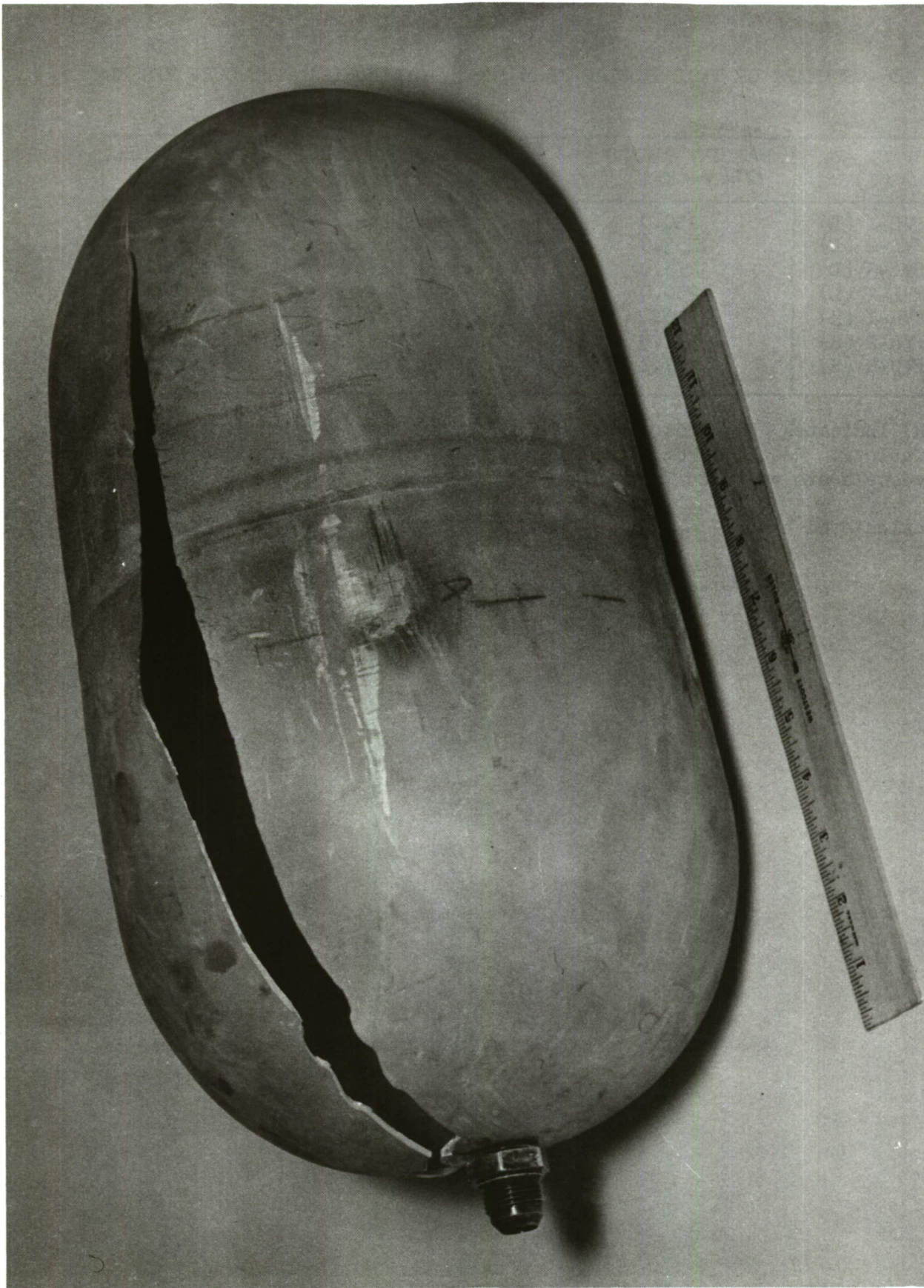
FIGURE 20 — FRACTURE PATTERN IN "LOW" STRENGTH 5CrMoV PRESSURE VESSEL — NO. PVL-1.
