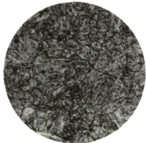
AS — SPUN MATERIAL ANNEALED AND THEN HEAT TREATED TO "HIGH" STRENGTH LEVEL
