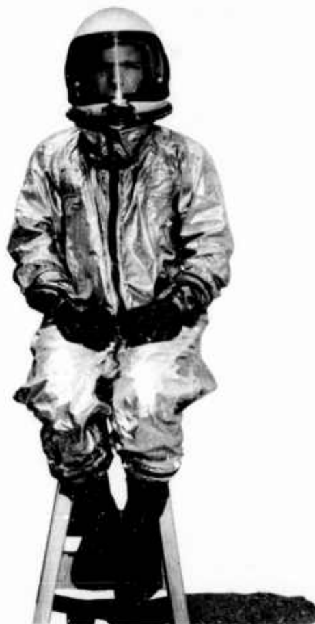
Fig.23 Modified MC-2 full-pressure suit
