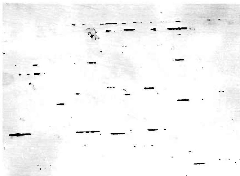
Figure 13. Photomicrograph of Case W-78, Illustrating Excessive Inclusions in Flash Weld. Case Failed at a Low Stress Level (239,200 psi). Magnified 100 Times
