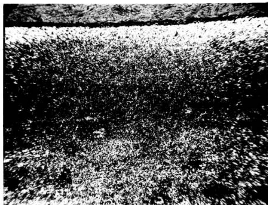
Case F-106. Heavy Decarburization. Magnified 100 Times
