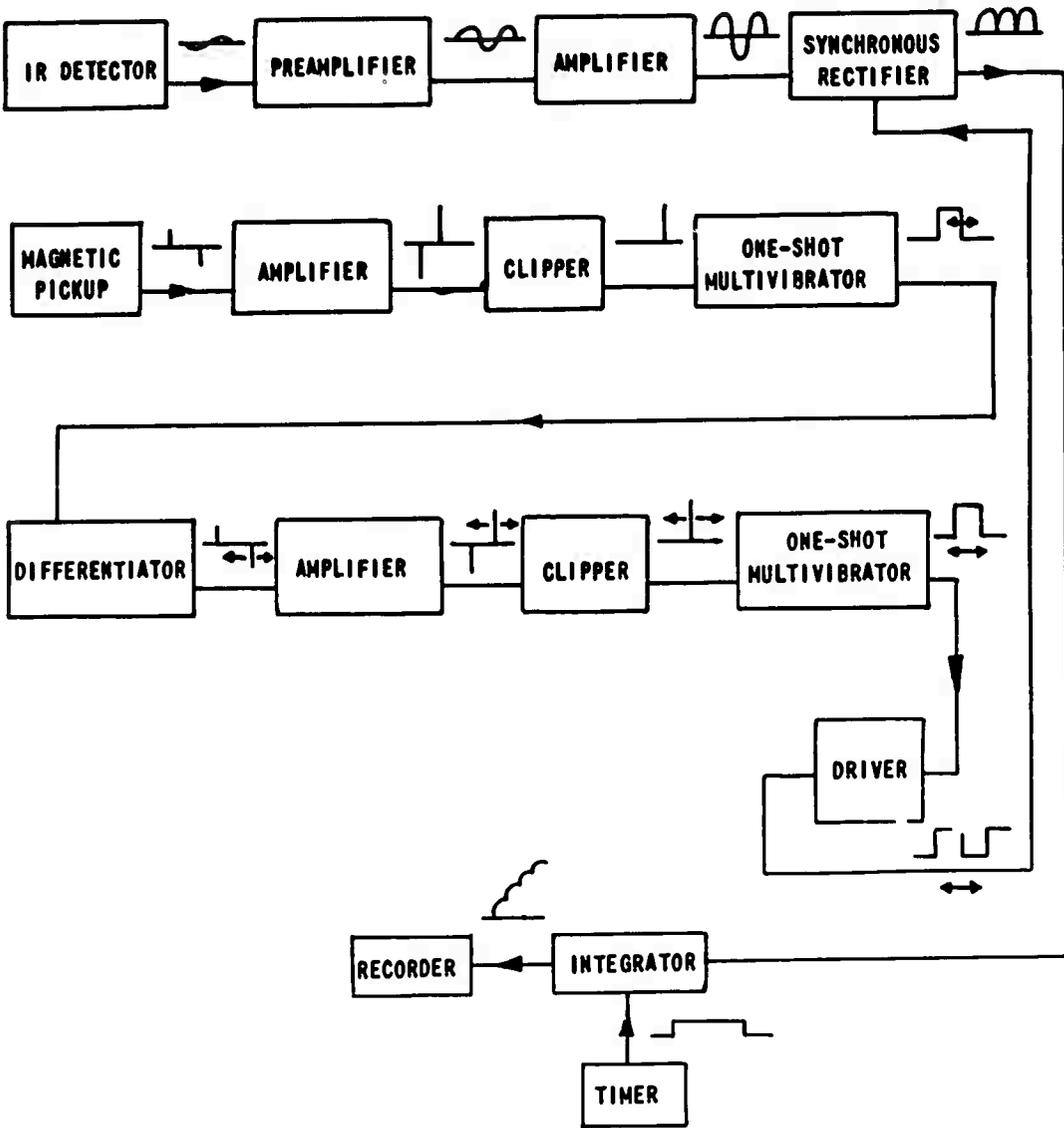
Figure 2. ELECTRONIC SYSTEM BLOCK DIAGRAM WITH WAVEFORMS
