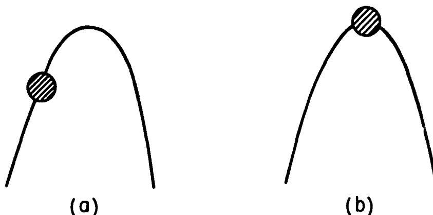
Fig. 17. Showing the effect of offsetting the antenna beam from the sun .
