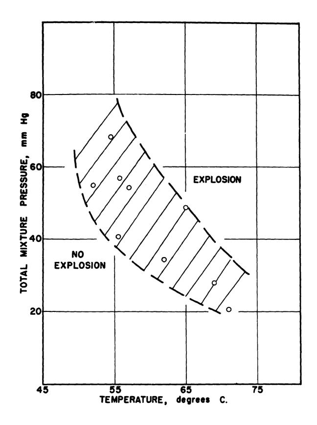
Explosion Region for Tetraborane-Oxygen-Helium Mixtures in the Ratio 1 to  $5^{3}/_{2}$  to  $5^{3}/_{2}$  in 6.8 cm Diameter Bulbs (Figure follows page 41.)
