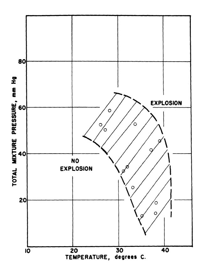
Explosion Region for Tetraborane-Oxygen Mixtures in the Ratio 1 to  $5^{3}/_{2}$  in 4.0 cm Diameter Bulbs
