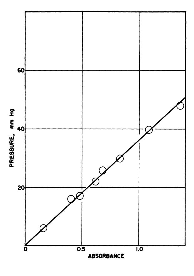
Infrared Absorbance vs Pressure Curves for Tetraborane and Diborane at 5.30  $\mu$  (1890 cm  $^{-1}$ ) in 9 cm Path Length
