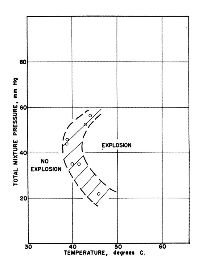
Explosion Region for Tetraborane-Oxygen Mixtures in the Ratio 1 to  $5^{1/2}$  in 6.8 cm Diameter Bulbs Packed with Glass Wool
