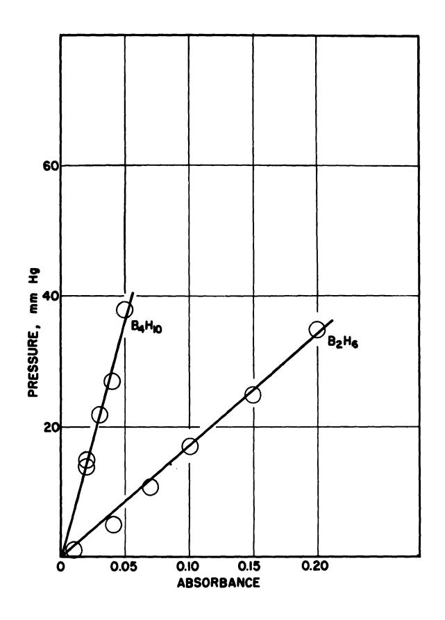
agreement and therefore a curve of absorbance versus pressure of partial oxidation product at 11.35 microns was constructed from them, as shown in Figure 7.
