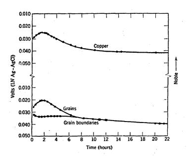
particular system of alloy and environment. However, it is important to realize that high reactivity is not a sufficient condition for cate phic failure. A certain amount of stress, directed across the reactive path, is also required. Stress Concentration
