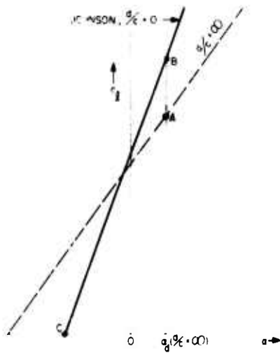
Fig. D6 - Effect of depth on lift coefficient - Johnson's method
