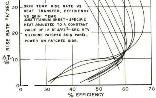
Figure 48. Efficiency Curves for Radiant Heat Method of Thermal Simulation. Titanium Sheet with Tension Patch Internal Heat Sink.
