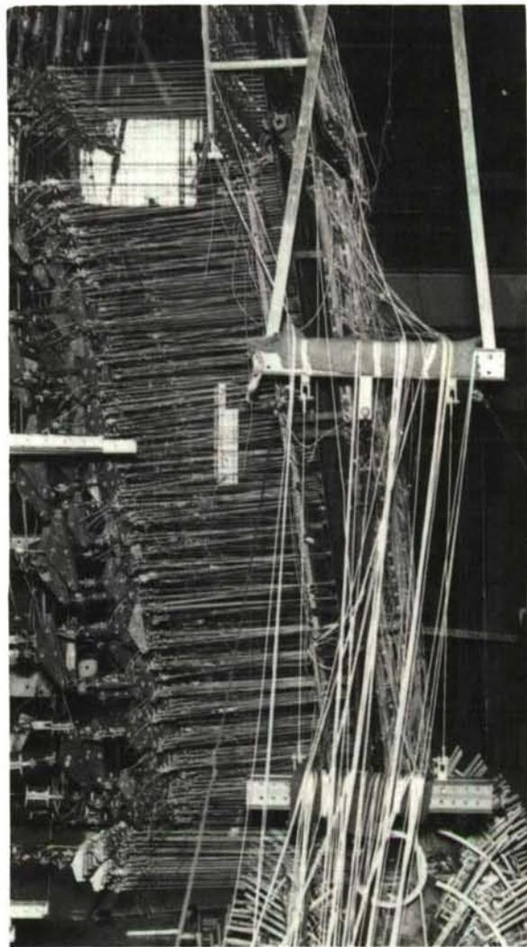
Figure 2A and 2B. B-58 Fin and Rudder Elevated Temperature Test Using RTV Silicone Bonded Tension Patches.
