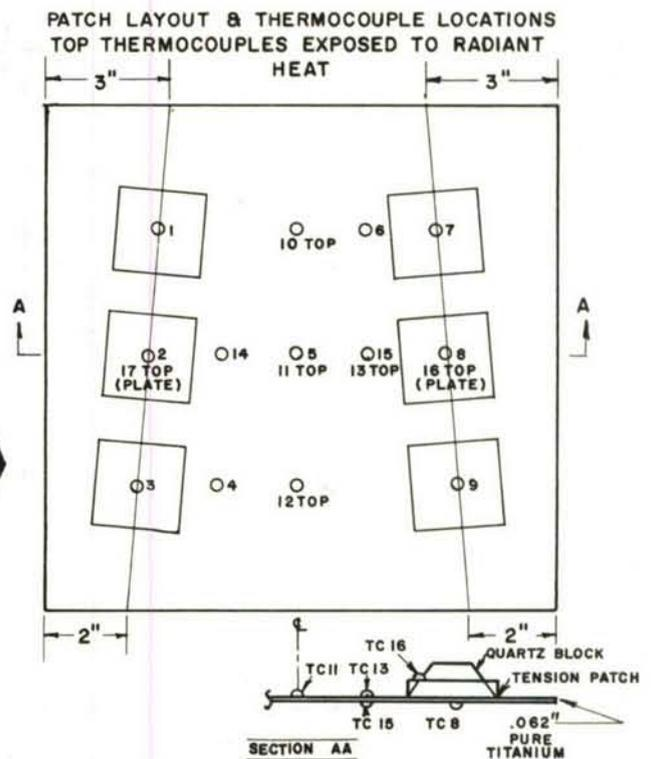
The efficiency of the system was calculated using constant power runs to the maximum calculated skin temperature at several temperature rise rates. All test specimens were sprayed with a graphite absorbent paint.
