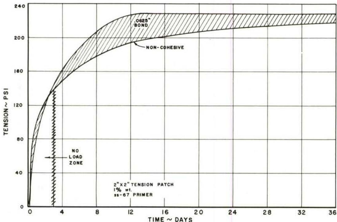
Figure 10. GE RTV 90 Silicone Bonded Tension Patch
