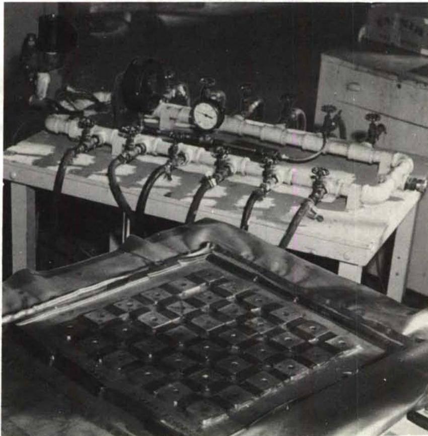
Figure 17. Vacuum Pressure Method for RTV Silicone Tension Patch Application
