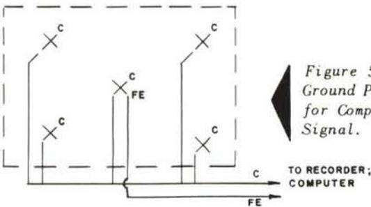
Figure 51. Thermocouple Single Ground Parallel Circuit Diagram for Computer Control Feedback Signal.
