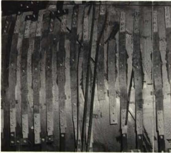
Figure 4. F-106 Engine Heat Test Using RTV Silicone Bonded Tension Patches and Shear Straps
