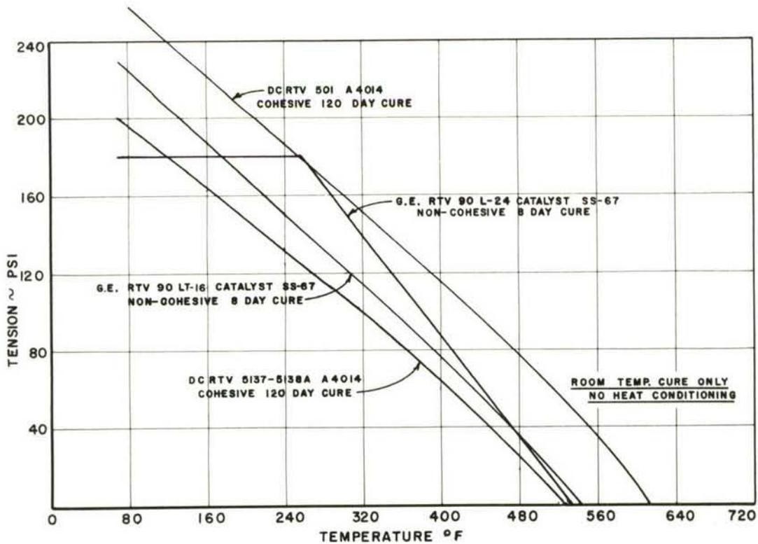
Figure 12. RTV Silicone Bonded Tension Patch Failing Load vs Test Temperature
