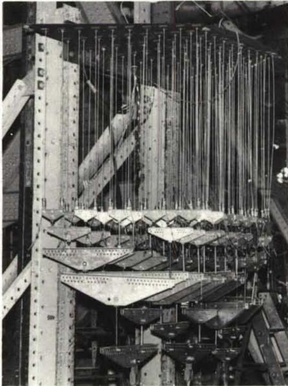
Figure 32. Titanium Missile Fin Test Set-up Using RTV Silicone Bonded Tension Patches. (Radiant Heat Reflectors Not Installed.)
