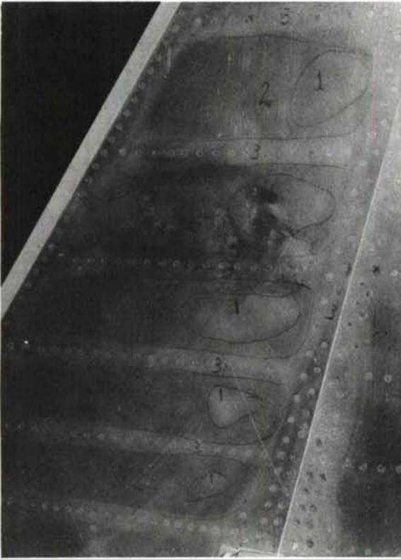
Figure 37. Titanium Missile Fin Oxidation.
