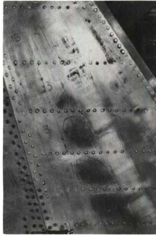
Figure 38. Titanium Missile Fin Oxidation.
