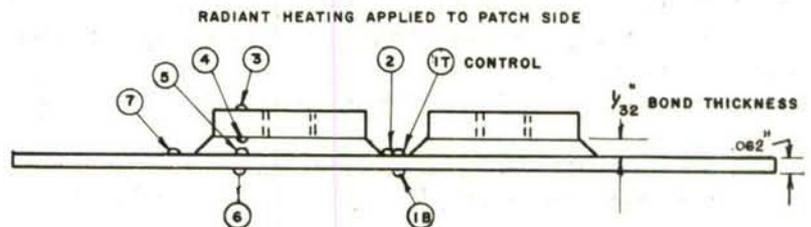
The test plates were made back to back (Fig. 31) and were then cut into individual test samples for curing and testing.
