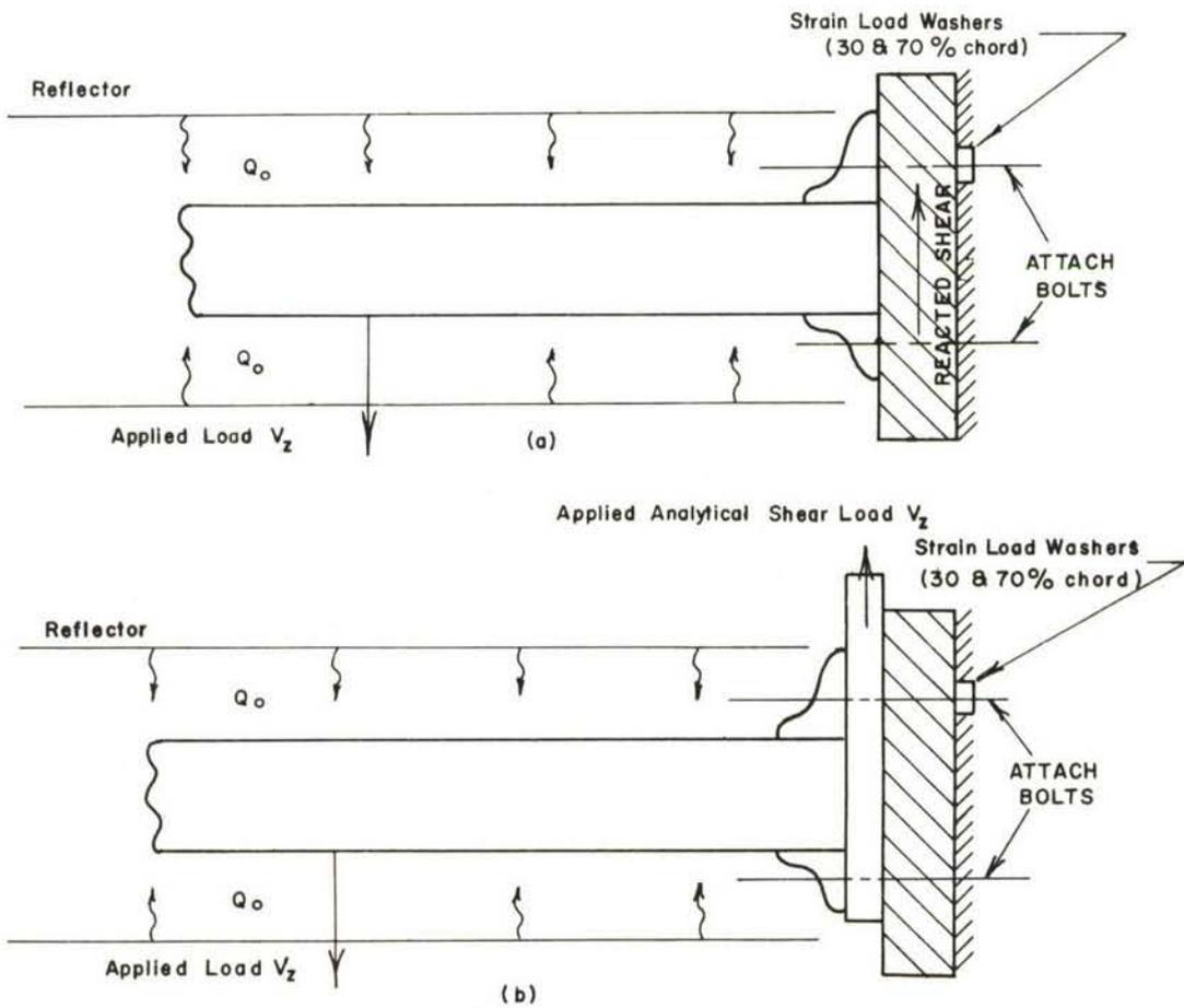
TENSION BOLTS TORQUED & CALIBRATED FOR COMPRESSION
