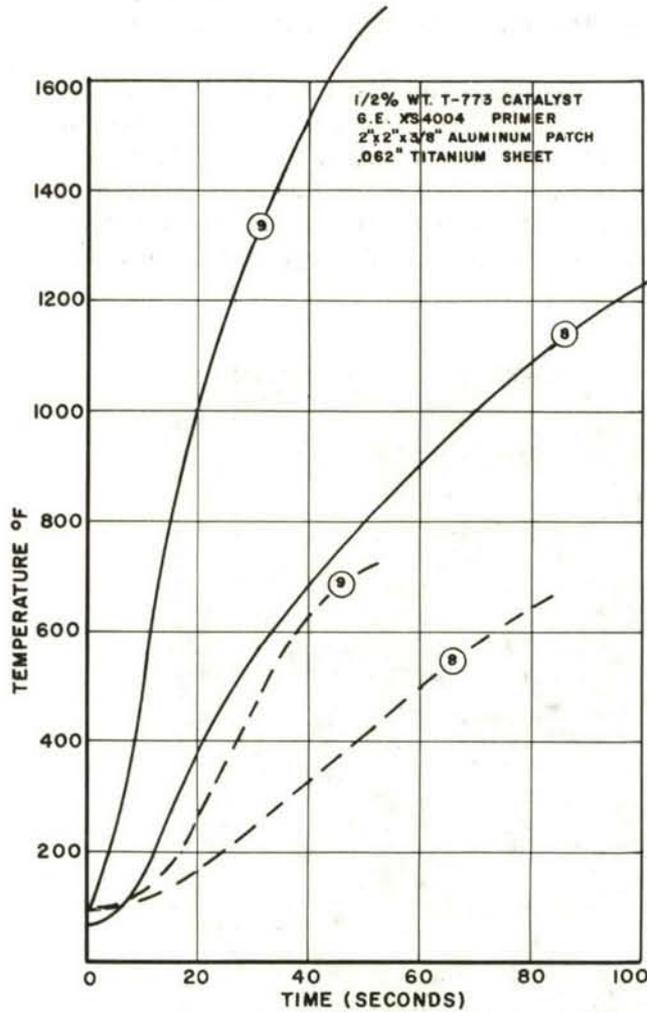
Figure 29. G.E. RTV 60 Silicone Bonded Tension Patch Panel Transient Heat Simulation to 2000° F. 50 psi Patch Load.
