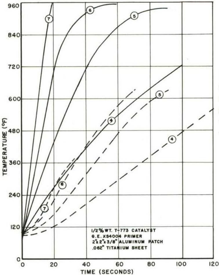
Figure 28 G.E. RTV 60 Silicone Bonded Tension Patch Panel Transient Heat Simulation to 1000° F. 50 psi Patch Load.
