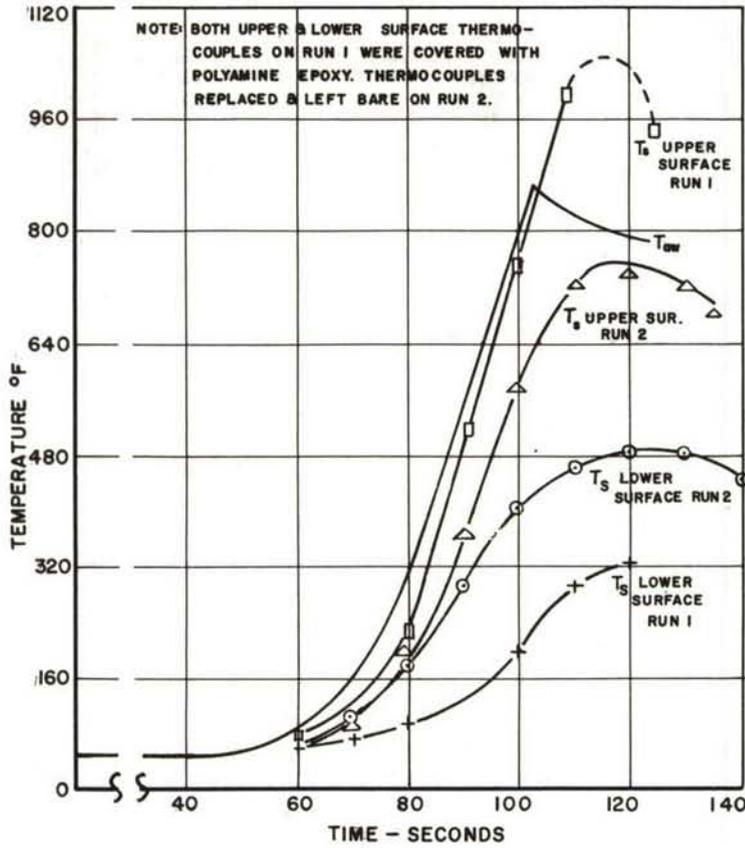
Figure 39A. Titanium Missile Fin Aerodynamic Temperature Simulation at 20 Per Cent Chord and 50 Per Cent Span
