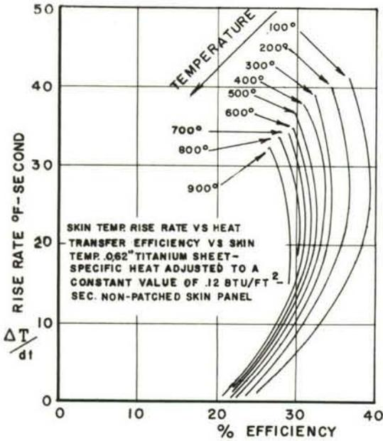
Figure 46. Efficiency Curves for Radiant Heat Method of Thermal Simulation. Titanium Sheet.
