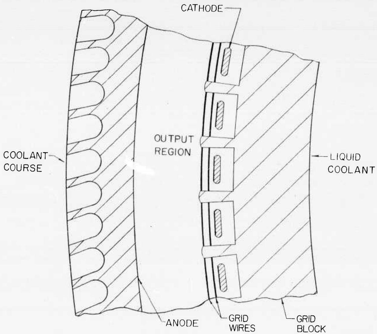
Figure 4 -- Axial Cross-Section of the Electronic Structure of the Model B Coaxitron
