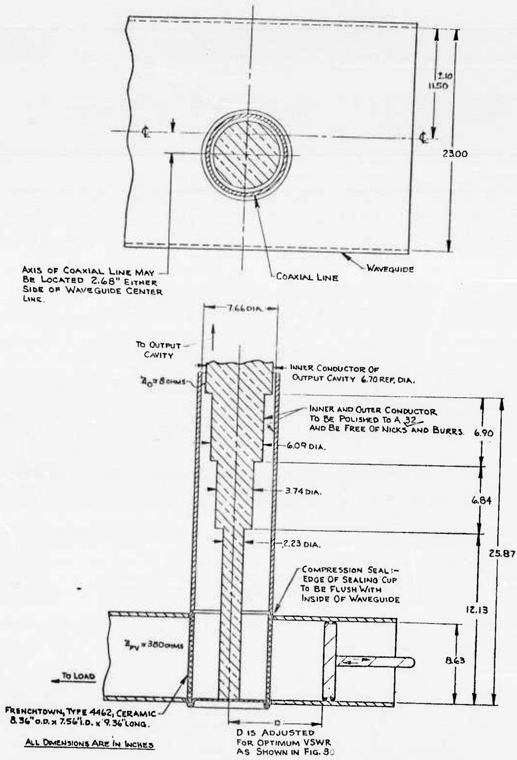
Figure 29 -- Dimensions of Interim Version, Model A Transition
