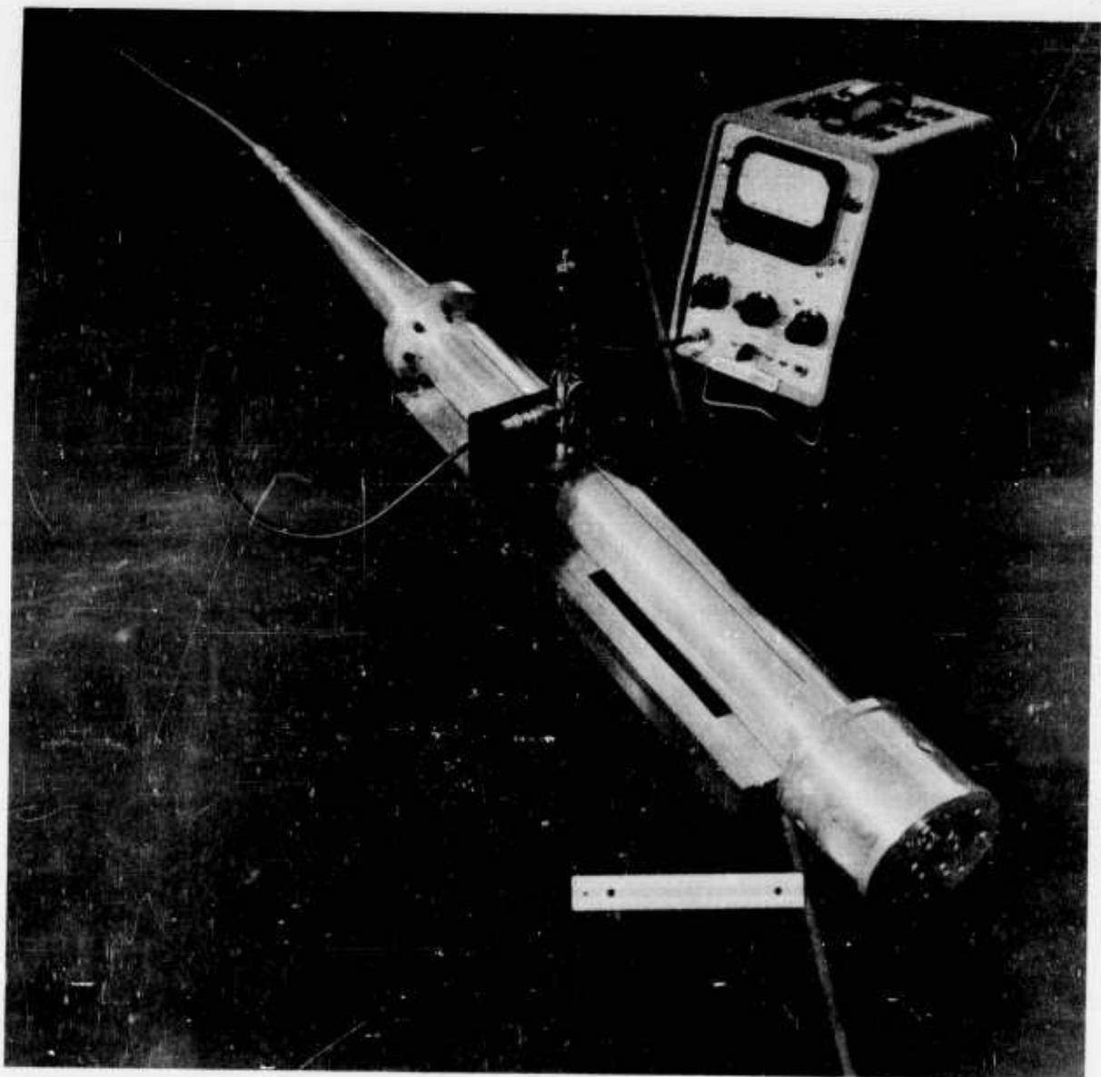
Figure 25 --- Scale Model Single-Tuned Cavity One-Third Size, Coaxial Slotted Line and Coaxial Transformer Shown Assembled (Scale is 6-1/2" long)
