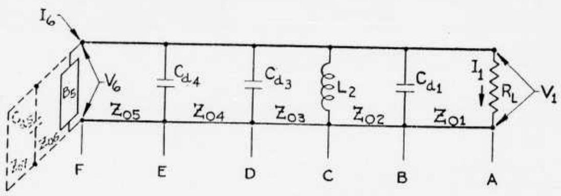
Figure 12 -- Equivalent Circuit for Configuration of Figure 11
