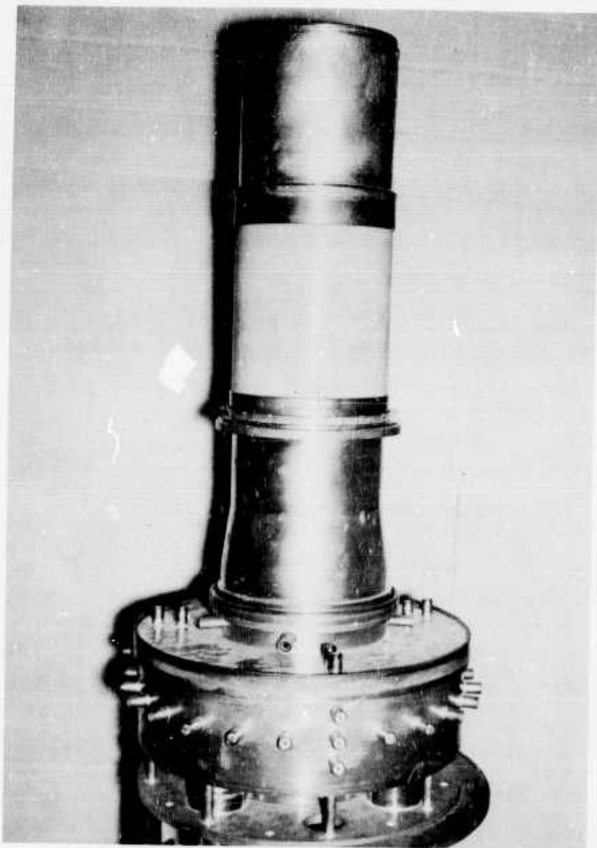
Figure 1 -- The Model B Coaxitron: The Larger Diameter at the Bottom Encloses the Anode, Grid Controlled Electronic Structure, and Most of the Rf Circuitry. The Small Cylinders Around the Periphery are the Voltage Sampling Probes. The Long Smaller Diameter Stack Encloses the Auxiliary Output Cavity and Coaxial Output Line. The Ceramic Cylinder at the Center of the Stack is the Output Vacuum Window for Coupling Rf Energy Directly to the Output Waveguide.
