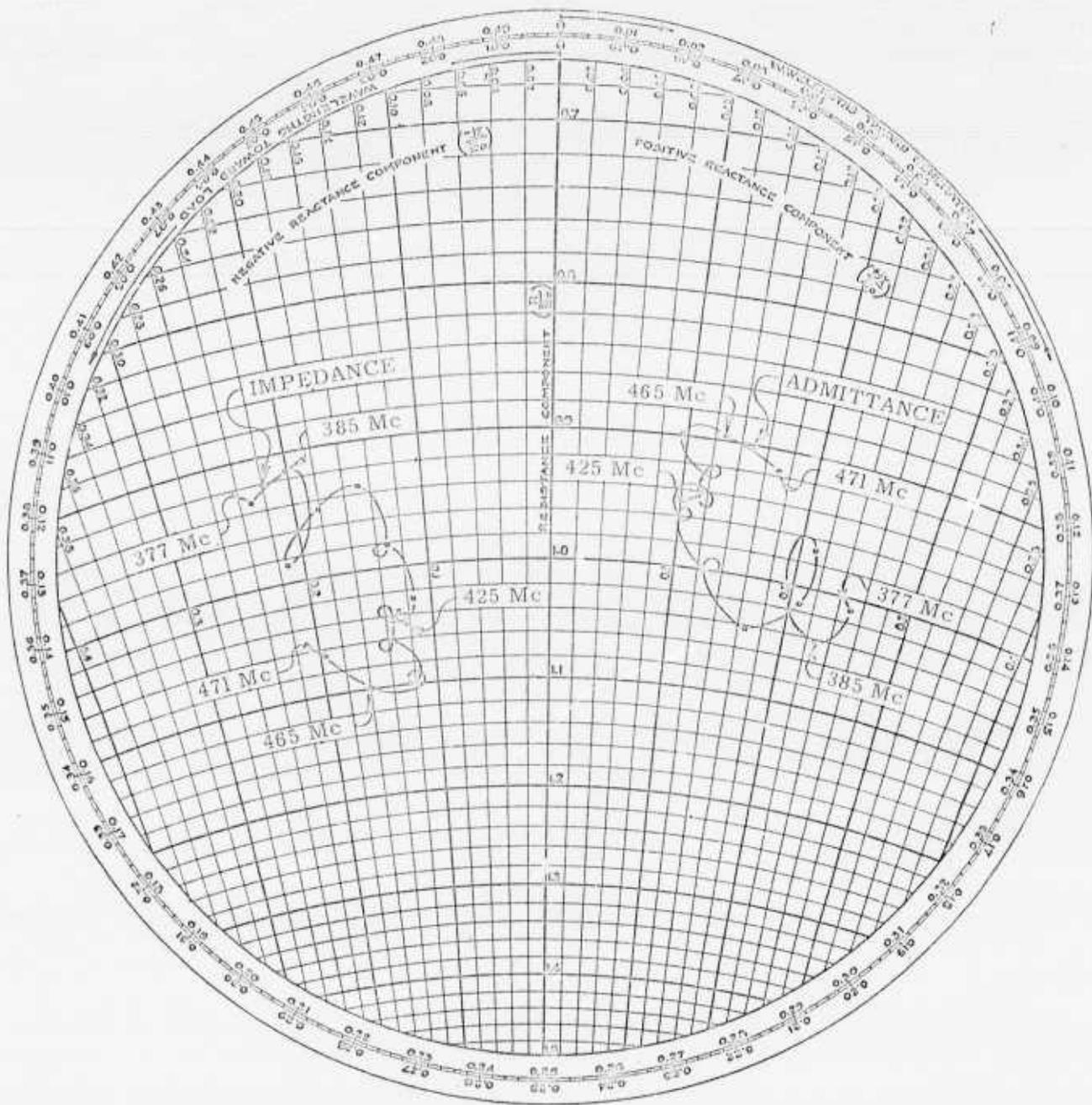
Figure 6 -- Normalized Impedance and Admittance vs. Frequency for the Model B Coaxitron Coaxial-to-Waveguide Transition.
