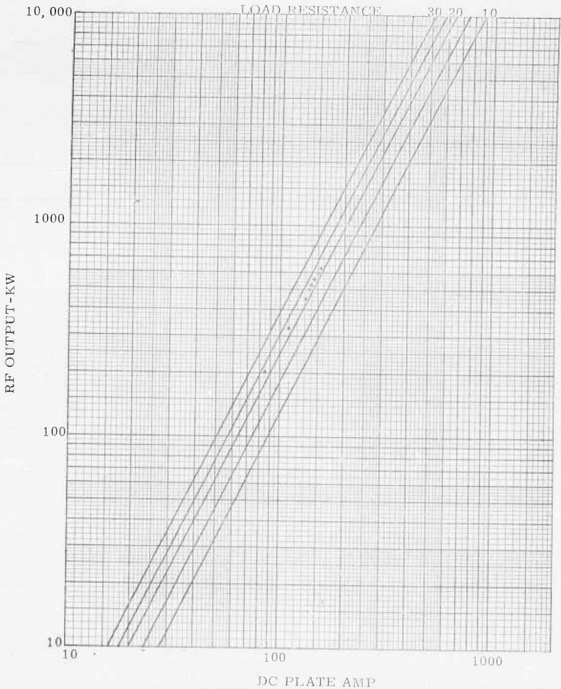
Figure 9 -- Class B Amplifier Performance: The Position of the Load Resistance Lines is set by Assuming  $I_{pRMS} = 1.1 I_B DC$ . The Points Plotted during Provisional Evaluation Establish a Load Resistance Line which when Extrapolated to 5,000 KW predicts a Plate Current of 450 Amperes. This Represents a Conservative Cathode Loading of only 5 Amperes per Square Centimeter.
