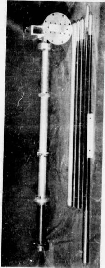
Figure 27 -- Adjustable Transition Shown Connected to Outer Conductor of the Slotted Line. In the Foreground are Various Size Lossy Tapered Inner Conductors, all of Which Taper from Some Higher Impedance to the Impedance of the Calibrated Load. These Tapers Were Used to Determine the Optimum Entrance Impedance to the Transition.
