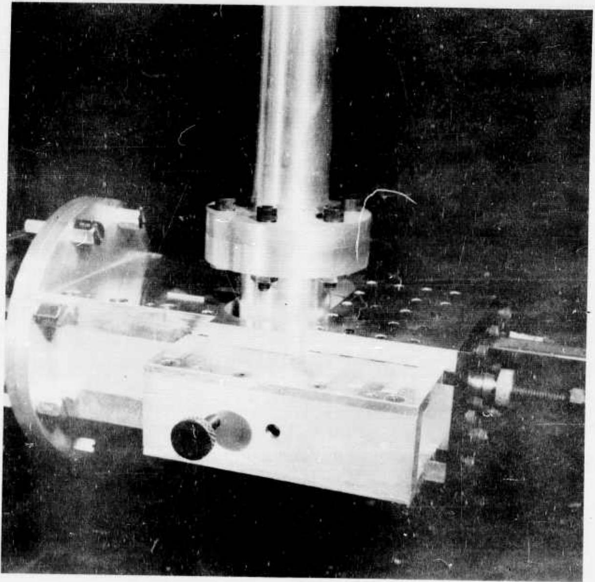
Figure 26 -- Side View of Scale Model Adjustable Waveguide-to-Coaxial Transition in 3.095" x 1.161" Waveguide, Showing Slide-Box Which Permits Adjustment of the Transverse Position of Coaxial Line in the Waveguide.
