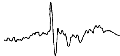
FIGURE 16. Oscillogram of single Canary motor. One cycle of a repeating wave. Fundamental frequency: 60 c; azimuth: 0 degree; distance: 1,000 ft.
