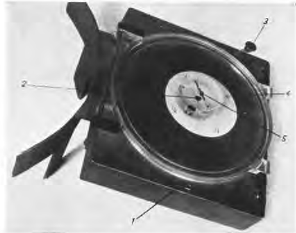
FIGURE 63. Top view of step-writer. (1) Thumb screw for orienting map paper, (2) knurled inking wheel, (3) plunger for distance input, (4) map paper, (5) compass needle.
