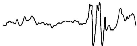
FIGURE 17. Oscillogram of single Canary motor. One cycle of a repeating wave. Fundamental frequency: 33 c; azimuth: 0 degree; distance: 1,000 ft.
