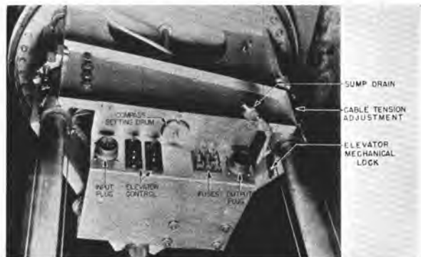
FIGURE 58. Elevator mechanism control panel in place.
