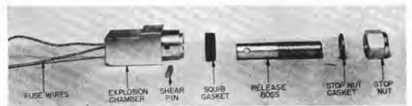
FIGURE 55. Squib bolt assembly parts.
