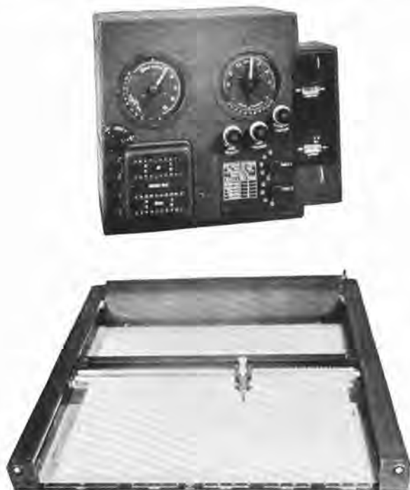
FIGURE 31. General view of airborne integrator and plotting table.
