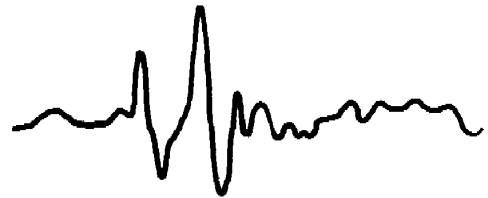
FIGURE 15. Oscillogram of single Canary motor. One cycle of a repeating wave. Fundamental frequency: 71 c; azimuth: 0 degree; distance: 1,000 ft.
