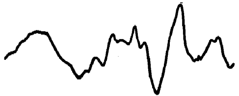
FIGURE 13. Oscillogram of BTL siren. One cycle of a repeating wave. Fundamental frequency: 230 c; azimuth: 0 degree; distance: 1,000 ft.
