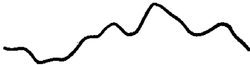
FIGURE 12. Oscillogram of BTL siren. One cycle of a repeating wave. Fundamental frequency: 470 c; azimuth: 0 degree; distance: 1,000 ft.
