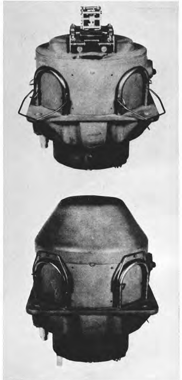
FIGURE 16. Inductor-type compass as developed for mounting in standard compass case. Upper , cover removed; lower , closed, as in use.
