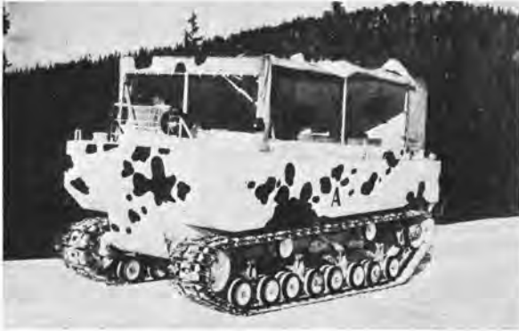
FIGURE 42. M-29 cargo carrier, equipped with odograph as used in winter tests at Camp Echo Lake, Colorado.
