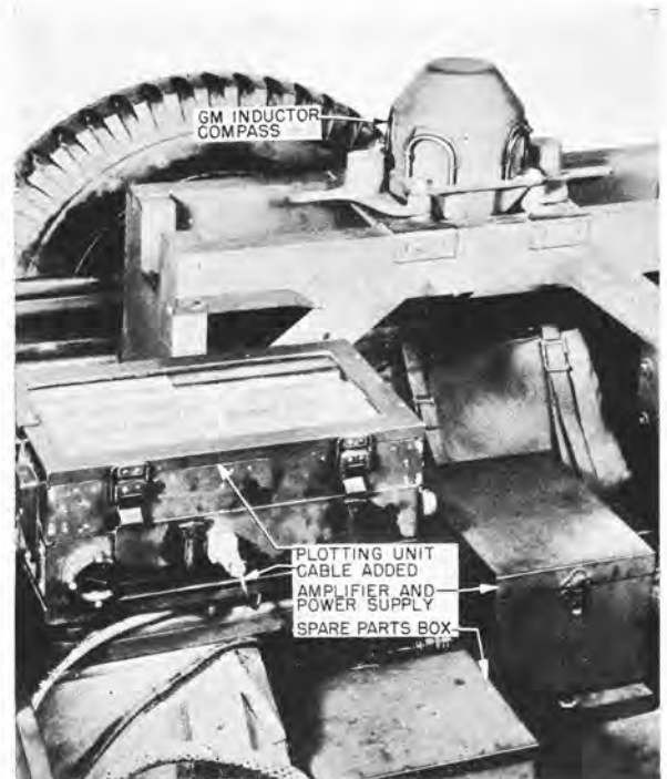
FIGURE 34. Installation of inductor compass on jeep, showing iron cylinders for quadrantal compensation.
