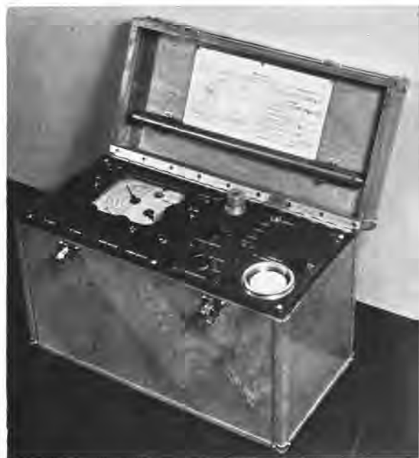
FIGURE 1. Radio chronometer comparator. The left-hand side of the cabinet is the radio receiver; the comparator dial is in the lower right-hand corner.
