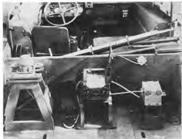
FIGURE 46. Odograph installation on amphibious truck (DUKW). Impeller in board (just forward of partition) for travel on land. Left, compass; center, plotting unit; right, log pickup unit.
