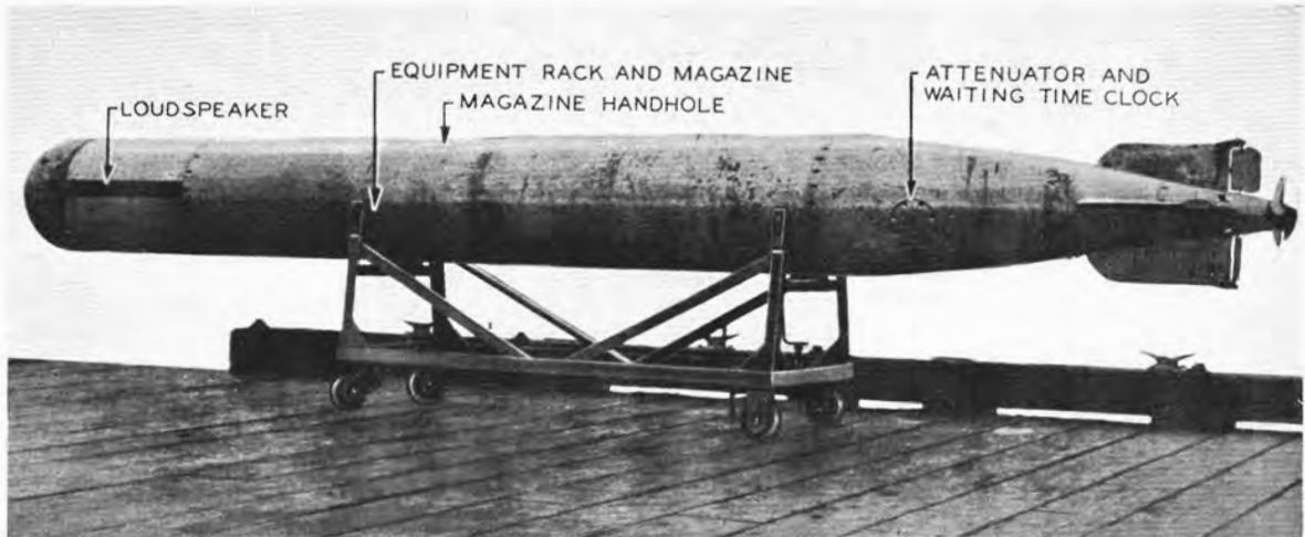
FIGURE 30. Water Heater prepared for firing.
