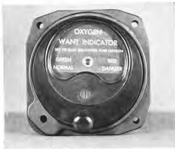
FIGURE 4. Signal light type oxygen want indicator.
