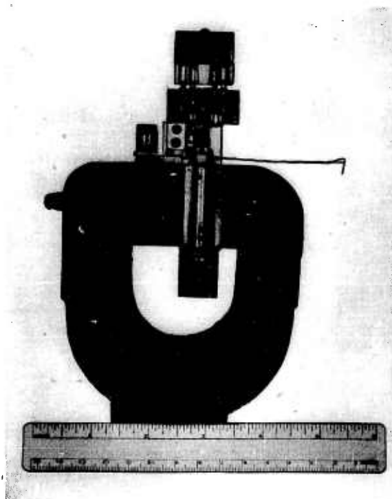
FIGURE 5. Galvanometer unit for dry paper recorder.
