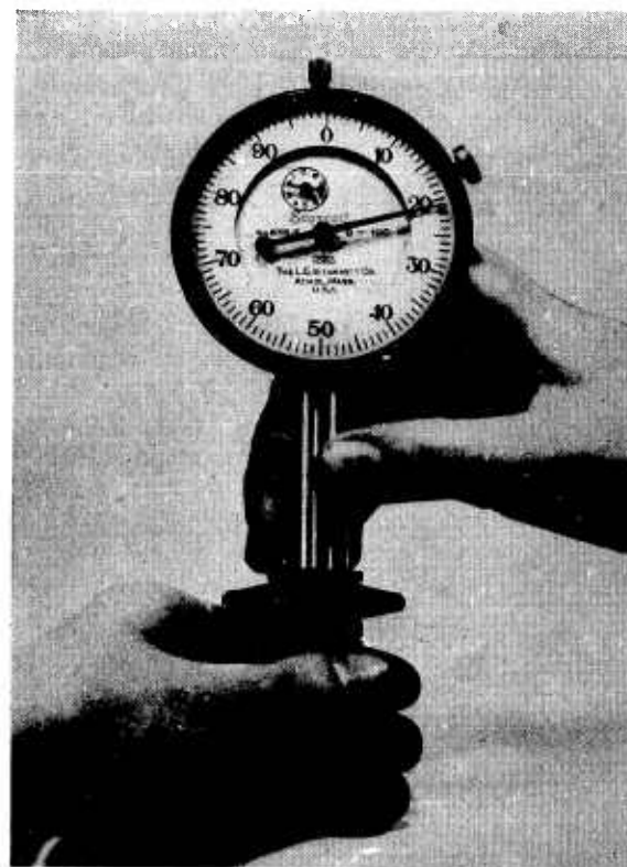
FIGURE 14. Measuring the deflection of the measuring pin with a dial gauge and adapter.
