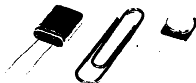
Figure 9. - Comparison of size of cased conventional and micro-module crystals.
