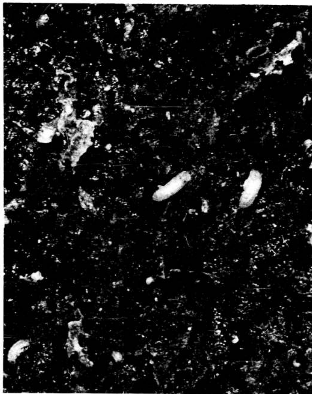
Figure 4. Linnoria crawling and burrowing on the surface of creosoted piling.
