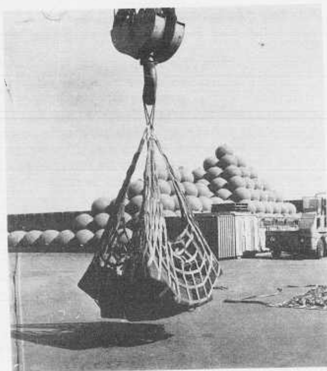
Fig. 7. - Static load test with 14,000 pound test load. NSRDF Neg. No. 293-22.
