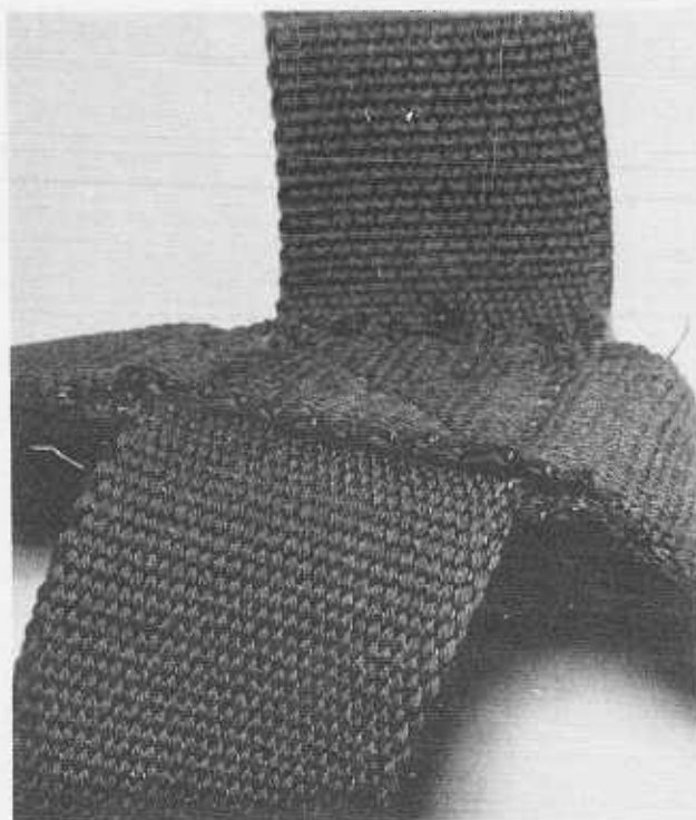
Fig. 2. - Enlarged view of the nylon slotted webbing. NSRDF Neg. No. 59-13.
