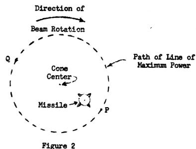
Cross-section of Cone with Observer Looking up the Cone (from antenna to target)
