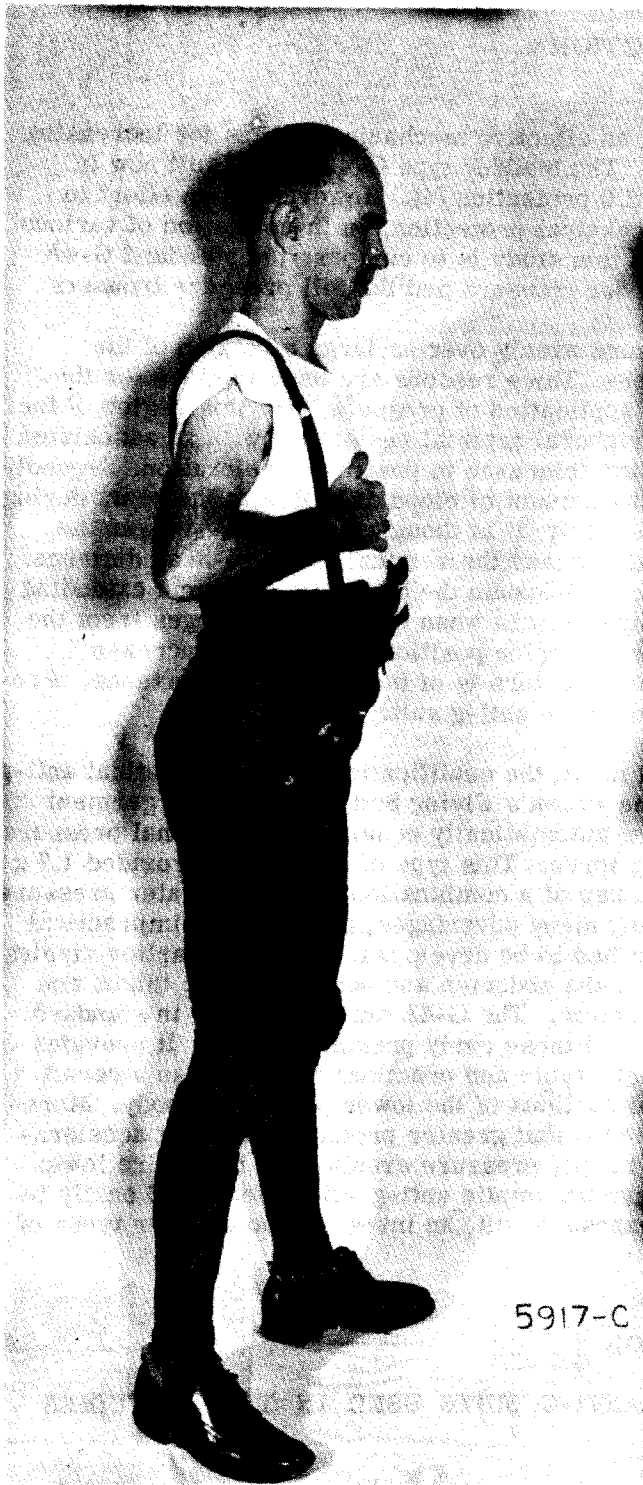
Figure 1 - Subject wearing the full pressure anti-g suit. In this particular model the outer reinforcing trousers were attached to the inner trousers and were adjusted to various sizes by the lacing on each leg.
