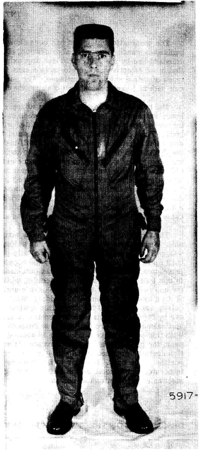
Figure 2 - Subject wearing the full bladder anti-g suit. The outer appearance is quite similar to the standard G-4A anti-g suit. The two inlets for pressurization are visible in this picture.
