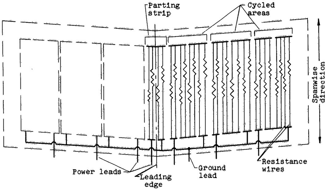
Figure 5. - Schematic diagram showing internal circuitry of boots.
