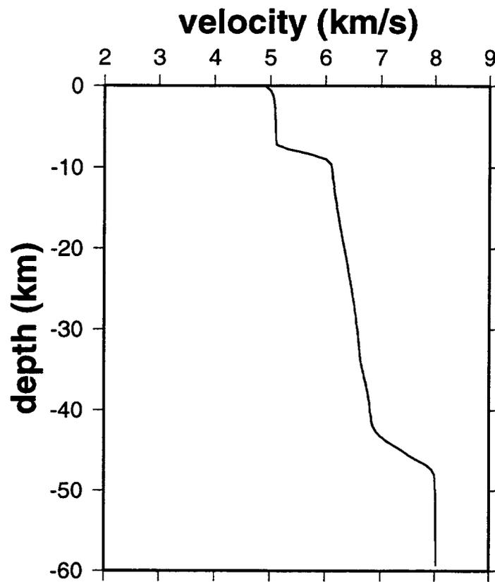
Figure 4. Reference (starting) 1-Dimensional model from Gao and Richards [1994].
