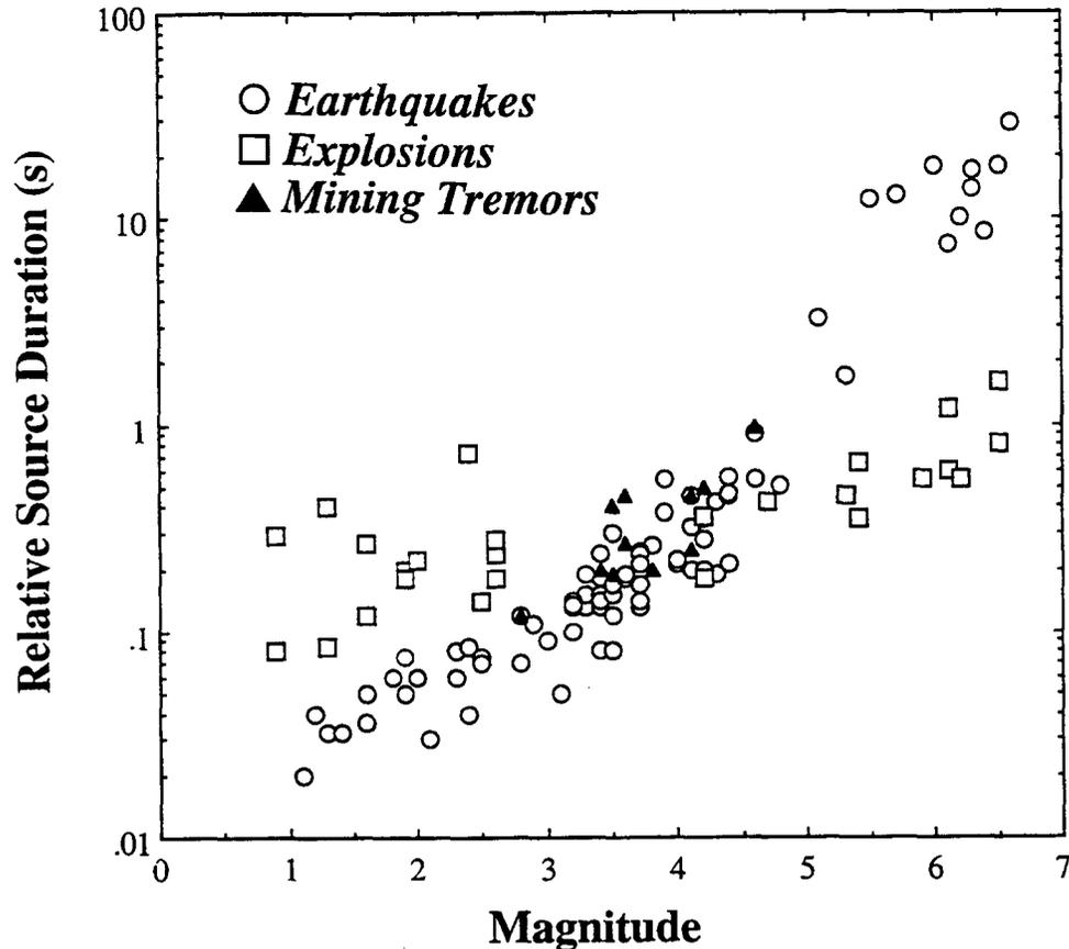
Figure 7: Source duration vs. magnitude for natural earthquakes (circles), explosions (squares), and mining tremors (filled triangles), determined by EGF analysis. For events having magnitude less than 2.5 or greater than 4.5, the source duration is a good discriminator between earthquakes and explosions. In the remaining magnitude range (2.5 to 4.5) the earthquake, explosion and mining tremor populations overlap.
