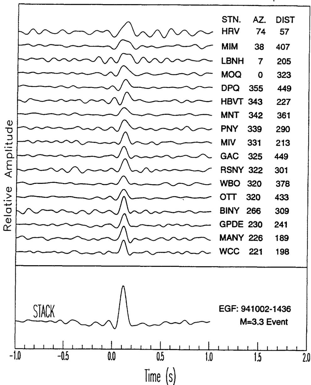
Figure 5: Estimated RSTFs of the 941002-1127 M=3.7 earthquake in central Massachusetts. Shown is the RSTF obtained at each of 17 stations together with the stack of the individual station estimates. The average source duration is about 0.15 s. The columns at the right show the code, azimuth and epicentral distance of each station. The variation of the source pulse width and amplitude with azimuth suggests that the rupture propagates to the southwest.
