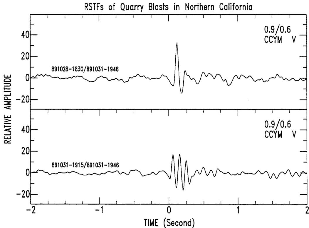
Figure 2: Estimated relative source time functions (RSTFs) of two small blasts ( $M=0.9$ ) in Kaiser Quarry, California. Both RSTFs were determined relative to the same EGF event. The date and time of each blast and the EGF event are labeled on the left part of each frame. The numbers on the right are the magnitudes of the event and EGF event.
