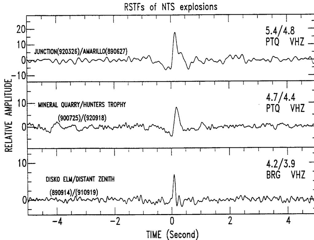
Figure 4: RSTFs of three nuclear explosions at the Nevada Test Site, determined from regional waveform data. The source durations of the explosions range from 0.35 to 0.65 s. The two bottom events are tunnel shots. Note the 'spall phase' of the explosions JUNCTION and DISKO ELM.
