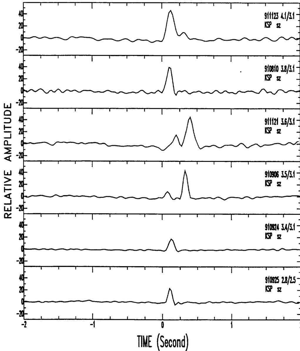
Figure 6: RSTFs of six mining tremors in Lubin, Poland. The magnitudes of the events range from 2.8 to 4.1. The source durations inferred from the RSTFs range from 0.15 to 0.6 s.
