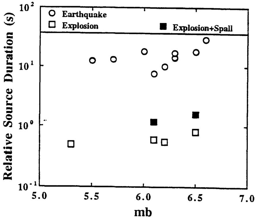
Figure 1: Comparison of source durations of earthquakes and nuclear explosions in central Asia. Source duration of EGF of each event was measured from its relative source time function, retrieved using the EGF method. (From Li et al., 1995.)
