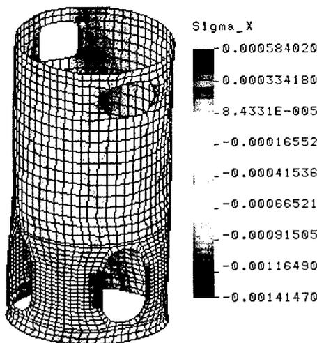
Fig. 7. Axial strains.
