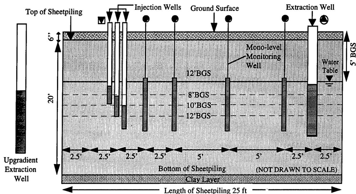
Figure 4. Cross section of a typical outside lane
