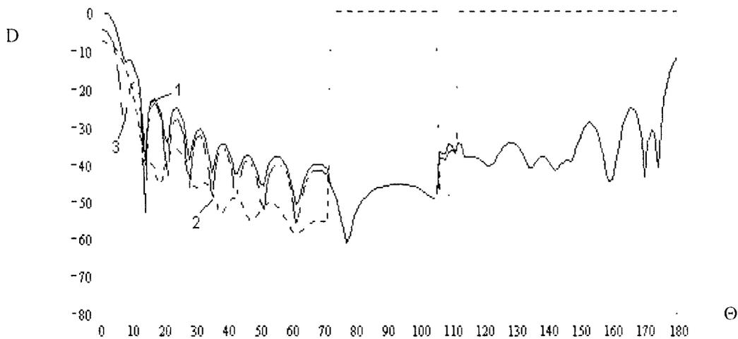
Fig. 2. The pattern of a reflector ( $f=1$  GHz)
